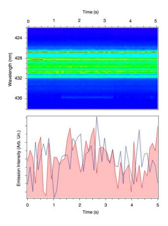
**Figure 4**. Competition between different modes in the Fabry-Pérot and random lasing cavity. (a) Temporal evolution of the lasing emission spectra above threshold (exemplary data from the P4 region, each spectrum is averaged over 10 laser shots). (b) Temporal evolution of the intensity of the lasing peaks at  $\lambda$ =426.7 nm (continuous line) and  $\lambda$ =428.2 nm (dotted line), respectively. Excitation fluence = 1.4 mJ cm<sup>-2</sup>.
