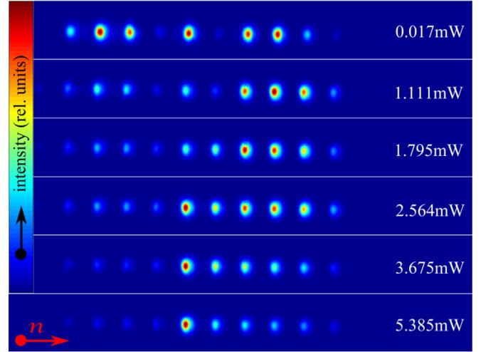
Fig. 3. Experimental output intensity distributions at different peak power levels illustrating the transition from Bloch oscillations to soliton formation. The corresponding calculated evolution dynamics is shown in Fig. 2. The red arrow indicates the direction of refractive index growth.
