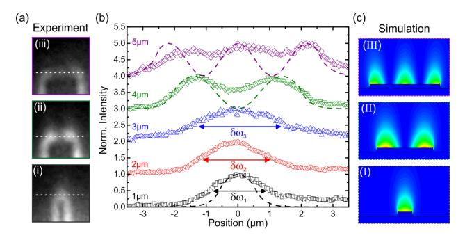
Figure 3 - (a) Spatially resolved quantum dot photoluminescence images for waveguide width (i)  $w_{WG} = 1 \ \mu m$ , (ii)  $w_{WG} = 4 \ \mu m$  and (iii)  $w_{WG} = 5 \ \mu m$ . (b) Extracted quantum dot intensity as a function of position at the remote waveguide end for waveguide widths  $w_{WG} = 1 \ \mu m$  (bottom) to 5  $\mu m$  (top). (c) Corresponding simulation of the plasmon mode for (I)  $w_{WG} = 1 \ \mu m$ , (II)  $w_{WG} =$ 4  $\mu m$  and (III)  $w_{WG} = 5 \ \mu m$ .
