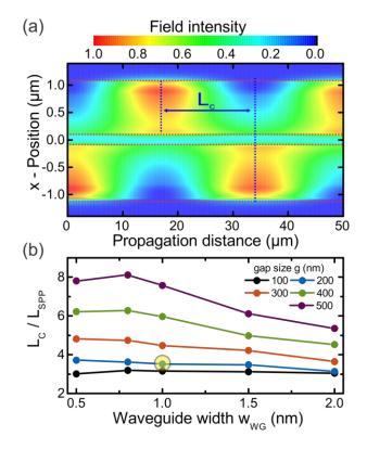
Figure 4 - (a) Simulation of the plasmonic mode profile as a function of propagation distance. (b) Ratio  $L_C/L_{SPP}$  as a function of  $w_{WG}$  for gap sizes g = 100 nm to 500 nm.
