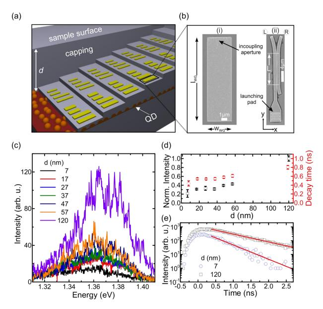
Figure 1 - (a) Schematic sample layout. (b) Scanning electron microscope images of (i) a plasmonic waveguide and (ii) a plasmonic beamsplitter. (c) Typical quantum dot micro-photoluminescence spectra recorded for different quantum dot-surface separations d. (d) Time-integrated (black) and time-resolved (red) micro-photoluminescence as a function of d. (e) Time-resolved transients for  $d = 7 \pm 4$  nm (blue circles) and  $d = 120 \pm 1$  nm (black squares).
