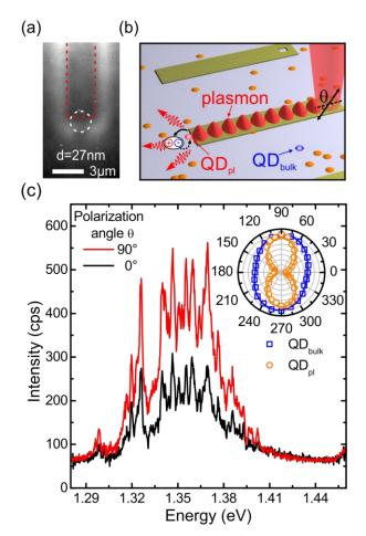
Figure 2 - (a) CCD camera measurement of the plasmonic waveguide imaged via the spectrally integrated QD signal. (b) Schematic excitation scheme of plasmon-excited quantum dots. (c) Polarization-resolved micro-photoluminescence spectra for  $\theta = 0^{\circ}$  (black) and  $\theta = 90^{\circ}$  (red). (Inset) Corresponding polar plot for plasmon-excited (orange) and bulk (blue) quantum dots.
