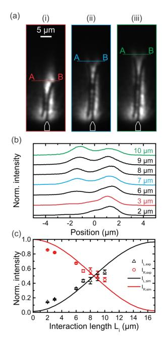
Figure 5 - (a) Spatially resolved quantum dot photoluminescence images for plasmonic beamsplitters with interaction length (i)  $L_i = 3 \mu m$ , (ii)  $L_i = 7 \mu m$  and (iii)  $L_i = 10 \mu m$ . (b) Cross-sectional intensity profiles for  $L_i = 2 \mu m$  (lower spectrum) to 10  $\mu m$  (upper spectrum). (c) Experimentally determined normalized output intensity (symbols) and comparison with simulation (solid lines).
