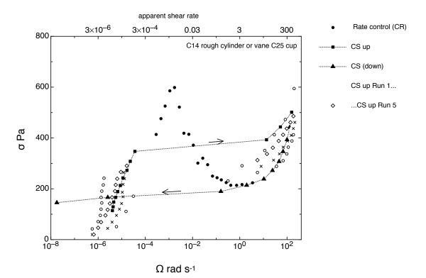
**Fig. 1.** Flow curves plotted as shear stress versus the angular velocity of the 14 mm diameter rotor. The corresponding, apparent Newtonian shear-rate is given on the upper ordinate for guidance purposes. Filled circles – controlled rotation rate. Connected filled squares – ascending staircase of controlled stress; connected filled triangles – descending. Remaining points – further examples of many runs in ascending controlled stress mode.
