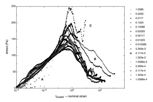
**Fig. 9** - As fig. 8 but with time multiplied by the apparent strain-rate to give the engineering or nominal strain.
