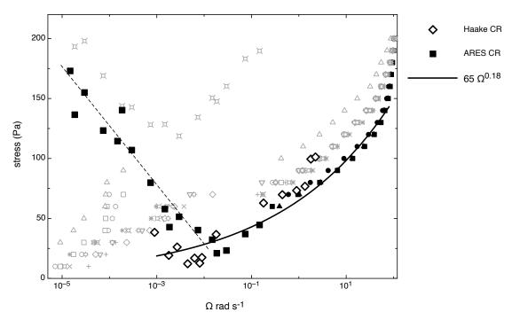
**Fig. 7** - As fig. 6 but with the CS up curves and the CR peak stress points greyed out for clarity. The higher shear branch is compared with a power-law up to the point where shear thickening sets in.
