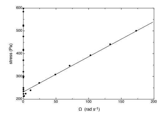
**Fig. 2**. The multi-valued flow curve suggested by fig. 1 plotted on a linear scale. The drawn line has a slope of 1.6 Pa.s  $rad^{-1}$ , which equates to an apparent plastic viscosity of ca. 0.55 Pa.s, based on the apparent Newtonian shear-rate, and hence a relative viscosity of > 500.
