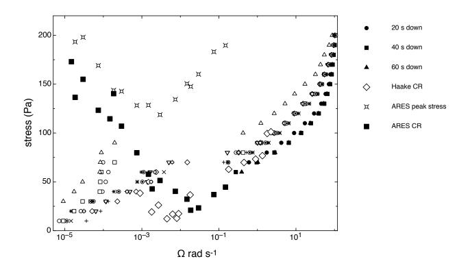
**Fig. 6** - Comparison of controlled stress with steady-state data from controlled-rate measurements. Also shown is the peak stress measured with ARES during flow-start-up. The vane diameters were 8.1mm (ARES), 24mm (Haake) and 28mm (AR-G2) and to compensate for this the rates for the ARES and the Haake have been scaled by factors of 8.1/28 and 24/28, respectively.
