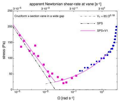
The total stress can be decomposed into solidphase and viscous parts.
