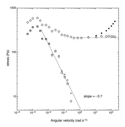
**Fig. 3** - Filled circles - the multi-valued flow curve suggested by fig. 1. Unfilled diamonds - the same data but with the viscous stress calculated using the plastic viscosity obtained from the linear plot show in fig.2. Unfilled squares and circles with the plateau stress subtracted, using values of 215 and 211 Pa, respectively.
