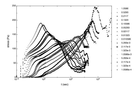
**Fig. 8** - Stress growth and decay at controlled strain-rate using the ARES. The parameter is the apparent mean (Newtonian) shear-rate and proportional to the angular velocity.
