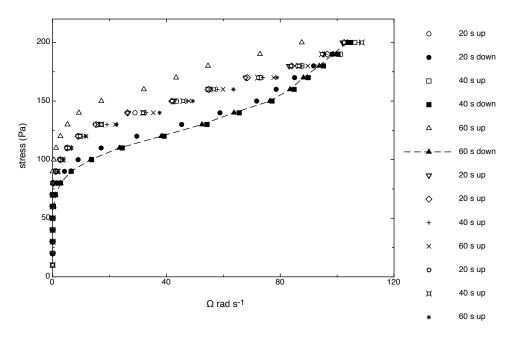
**Fig. 4** - Flow curves from controlled stress for three different dwell times per point. The filled points denote the down-curves. The hysteresis was not overtly time-dependent and thus not a manifestation of thixtropy in the usual sense.
