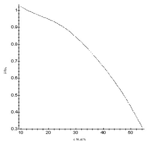
Fig. 5. Concentration dependence of an average 'atomic' magnetic moment,  $\overline{\mu}$ , of Ni-Fe alloy (with  $L1_2$ -type superstructure) at  $T_K(c_{Fe})$ .
