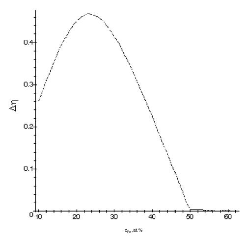
Fig. 2. Calculated theoretical dependence of long-range order parameter jump,  $\Delta \eta$ , of  $L1_2$ -type superstructure on Fe content,  $c_{\rm Fe}$ , at corresponding Kurnakov temperatures for f.c.c.-Ni–Fe alloy.
