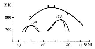
Fig. 6. Numerically calculated by cluster variation method dependencies of Curie (solid line) and Kurnakov (dotted line) temperatures on Ni content for f.c.c.-Ni-Fe alloys [14]; black circles—experimental points [9].
