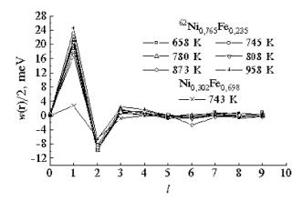
Fig. 1. Variation of 'mixing' energy  $w(\mathbf{r})$  with number of co-ordination shell l at different annealing temperatures for f.c.c-Ni-Fe alloy (within the approximation  $w(\mathbf{r})|_{\mathbf{r}=0}=0$  and without taking into account atomic size mismatch effects) [7].
