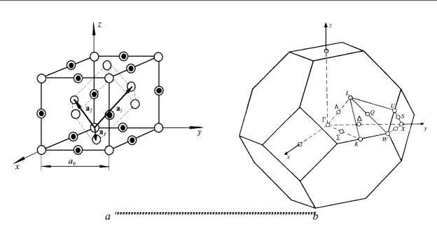
Fig. I.1. Conditional cubic (large cube) and primitive (interior small parallelepiped) unit cells (*a*), and the first Brillouin zone (*b*) of the Bravais f.c.c. lattice (in Fig. I.1*a*, O—sites, O—octahedral interstices,  $\{a_1, a_2, a_3\}$ —the basis vectors; in Fig. I.1*b*,  $\{\Gamma, X, W, L, K(U)\}$ —high-symmetry points,  $\{\Delta, \Lambda, \Sigma, Q, S\}$ —high-symmetry directions in *BZ*).
