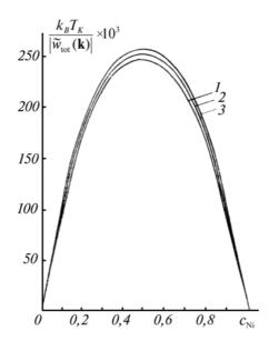
Fig. III.6. Kurnakov's point dependence on  $c_{\text{Ni}}$  for substitutional f.c.c.-Ni–Fe subsystem with different values of  $c_{\text{C}}$  and for  $\mathbf{k} = \mathbf{k}_X$  where  $|\omega_{\text{FeNiC}}(\mathbf{k}_X)| \approx 0.8 (1-c_{\text{C}} = 0, 2-c_{\text{C}} = 0.05, 3-c_{\text{C}} = 0.1)$ .
