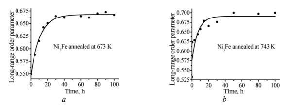
Fig. III.3. Time dependence of long-range order parameter for  $L_{1_2}$ -type Ni<sub>3</sub>Fe alloy; •—experimental data [107] for different temperatures: 673 K (a), 743 K (b).
