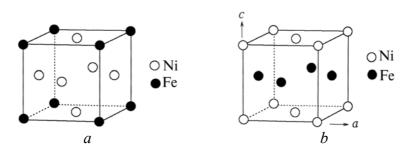
Fig. II.1. Ni<sub>3</sub>Fe  $L_{1_2}$ -type (*a*) and NiFe  $L_{1_0}$ -type (*b*) superstructures based on f.c.c. lattice. At low *T*, the layered NiFe superstructure may have the tetragonally-distorted unit cell with non-equal parameters, *c* and *a* (however,  $c/a \cong 1$ ).
