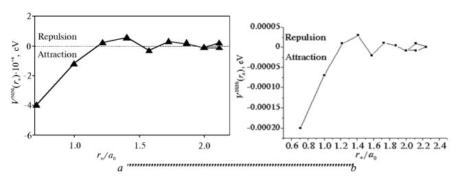
Fig. I.3. Dependence of the Ni–Ni strain-induced interaction energies on discrete site–site reduced distance  $r_n/a_0$  (n = I, II, ...) between Ni atoms within  $\gamma$ -Fe: based on [24] (a) and present work (b).
