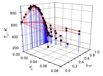
Fig. II.4. Experimental dependence ('circles' [67–87]) of Curie temperature,  $T_C$ , for f.c.c.-Ni–Fe alloy on the Fe concentration,  $c_{\text{Fe}}$ , and interstitial-impurity (C) concentration,  $c_C$ .
