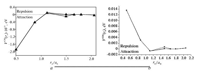
Fig. I.4. Dependence of the strain-induced interaction energies between C and Ni atoms on discrete interstice–site reduced distance  $r_n/a_0$  (n = I, II, ...) within  $\gamma$ -Fe: from [24] (a) and present work (b).
