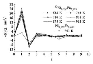
Fig. III.5. Variation of 'mixing' energy  $w_{tot}(\mathbf{r})$  with a number of co-ordination shell *l* for different annealing temperatures in f.c.c.-Ni–Fe alloys (within the postulated calibration equation  $w_{tot}(\mathbf{r})|_{\mathbf{r}=0}=0$ , and without explicit consideration of the strain-induced effects) [100].
