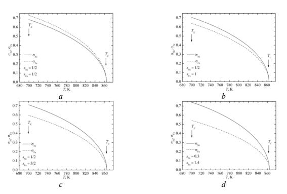
Fig. II.3. Temperature dependences of relative magnetizations,  $\sigma_{Ni}$  and  $\sigma_{Fe}$ , at different spin numbers of Fe and Ni atoms,  $s_{Fe}$  and  $s_{Ni}$ , in disordered f.c.c.-<sup>62</sup>Ni<sub>0.765</sub>Fe<sub>0.235</sub> alloy. For this content, an estimated value of the Curie temperature is as follows:  $T_C \cong 865$  K.
