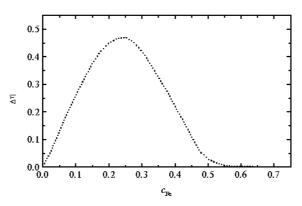
Fig. III.1. Calculated dependency of the jump of long-range order parameter,  $\Delta \eta$ , at  $T_K = T_K(c_{\text{Fe}})$  on the Fe content,  $c_{\text{Fe}}$ , for the disordering f.c.c.-Ni–Fe alloy with  $L_{12}$ -type (Ni<sub>3</sub>Fe) structure.
