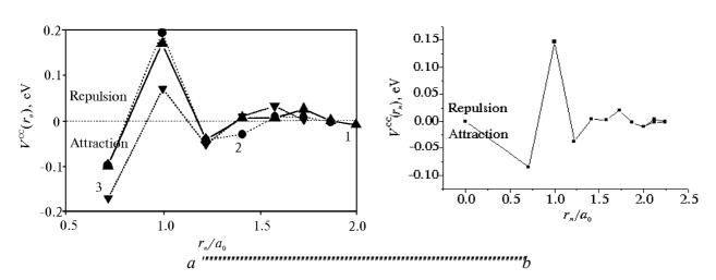
Fig. I.2. Dependence of the energies of C–C strain-induced interaction on discrete interstice–interstice reduced distance  $r_n/a_0$  (n = I, II, ...) between C atoms within  $\gamma$ -Fe [24, 25] (1),  $\alpha$ -Ni [17, 24, 25] (2),  $\gamma$ -Fe [28] (3)—(a), and within  $\gamma$ -Fe (present work)—(b).
