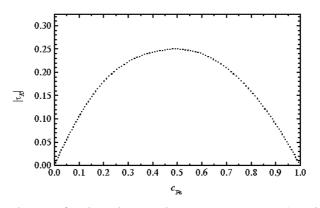
Fig. III.2. Calculated dependence of reduced Kurnakov's temperature (modulo),  $|\tau_K|$ , for the 1-st kind  $A1-L1_2$  transformation on the Fe content,  $c_{\text{Fe}}$ , in f.c.c.-Ni–Fe alloy.
