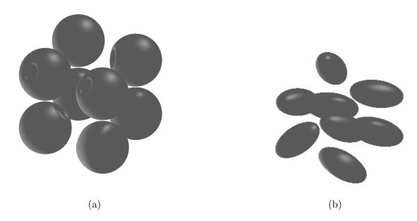
FIGURE 5. (a) Domain contains 8 bowl-shaped cavities. Distance between any two cavities is 0.5. (b) Domain contains 8 randomly oriented ellipsoids. Distance between any two ellipsoids is 0.05.
