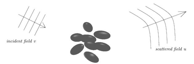
FIGURE 1. Geometry of scattering problem. An incident field v propagates in a medium with constant wave-speed and hits a scattering surface  $\Gamma = \bigcup_{p=1}^{m} \Gamma_p$  (shown for m=8). A charge distribution  $\sigma$  is induced on the surface  $\Gamma$  and generates an outgoing field u.
