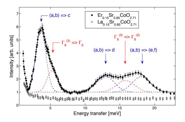
FIG. 3. (Color online) Energy spectra of neutrons scattered from  $Er_{0.15}Sr_{0.85}CoO_{2.71}$  and  $La_{0.15}Sr_{0.85}CoO_{2.71}$  at T=10 K. The data were taken with use of the TOF spectrometer KDSOG for moduli of the scattering vector 1.6<Q<3.3 Å<sup>-1</sup>. The lines denote Gaussian fits as explained in the text. The arrows mark the crystal-field transitions according to Fig. 2.
