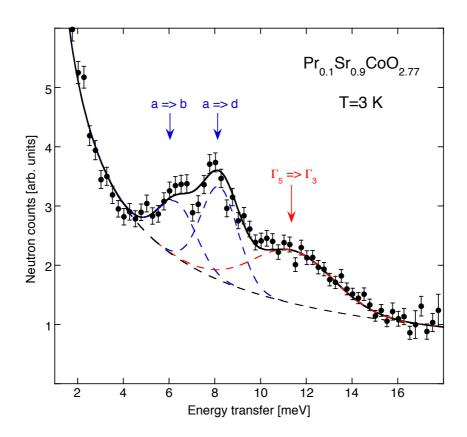
FIG. 7. (Color online) Energy spectrum of neutrons scattered from  $Pr_{0.10}Sr_{0.90}CoO_{2.77}$  at T=3 K. The data were taken with use of the TOF spectrometer CNCS for moduli of the scattering vector 1.5<Q<2.5 Å<sup>-1</sup>. The incoming neutron energy was 20 meV. The lines denote Gaussian fits on top of a power-law background as explained in the text. The arrows mark the crystal-field transitions according to Fig. 8.
