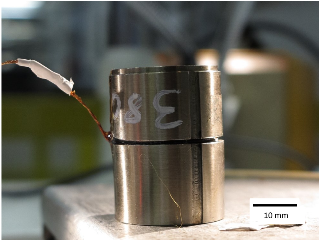
Figure 1. The assembled stack of two GdBCO bulk samples, each of diameter 24.15 mm and height 15 mm. The samples were reinforced with a ring of 3 mm thickness fabricated from 304 Stainless Steel. The recess visible in the ring served to accommodate the measurement wiring. The two bulk samples were then assembled into a stack with an array of 5 Hall probes at their interface using STYCAST thermally conductive epoxy resin. The Hall probes were arranged evenly in a line across the sample at -8 mm, -4 mm, 0, 4 mm and 8 mm from the sample centre.
