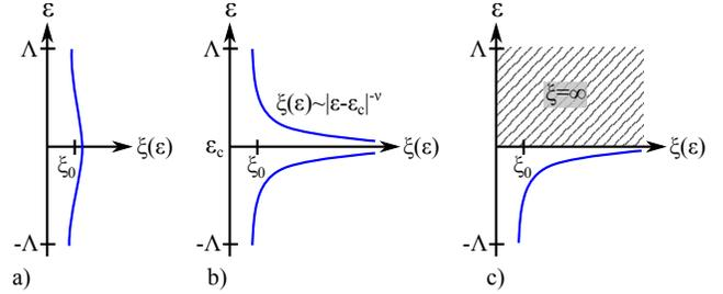
FIG. 1. Schematic dependence of SP localization length  $\xi$  on single-particle energy  $E$  for a fully-localized system (a), marginally localized system (b), and extended system with a mobility edge (c).
