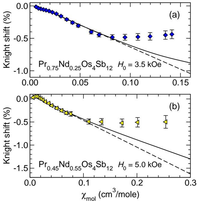
FIG. 9. (Color online) Clogston-Jaccarino plots of Knight shift  $K$  versus molar susceptibility  $\chi_{\text{mol}}$  for  $\text{Pr}_{1-x}\text{Nd}_x\text{Os}_4\text{Sb}_{12}$ . (a)  $x = 0.25$ . (b)  $x = 0.55$ . Data (symbols) from Fig. 6. Solid curves:  $K_{\text{av}}$  from Eq. (5). Dashed lines: linear fits for  $\chi_{\text{mol}}$  in range 0.01–0.05  $\text{cm}^3/\text{mole}$ .
