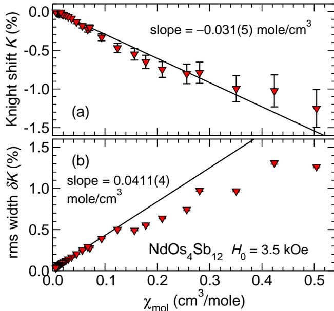
FIG. 4. (Color online) (a) Clogston-Jaccarino plot of  $\mu^+$  Knight shift  $K$  vs molar susceptibility  $\chi_{\text{mol}}$  in  $\text{NdOs}_4\text{Sb}_{12}$ . Line: linear fit for  $\chi_{\text{mol}}$  in the range  $0.01\text{--}0.05\text{ cm}^3/\text{mole}$ . (b) rms width  $\delta K$  of Knight shift distribution vs  $\chi_{\text{mol}}$ . Lines: linear fits to points for  $\chi_{\text{mol}}$  between  $0.01$  and  $0.05\text{ cm}^3/\text{mole}$ .
