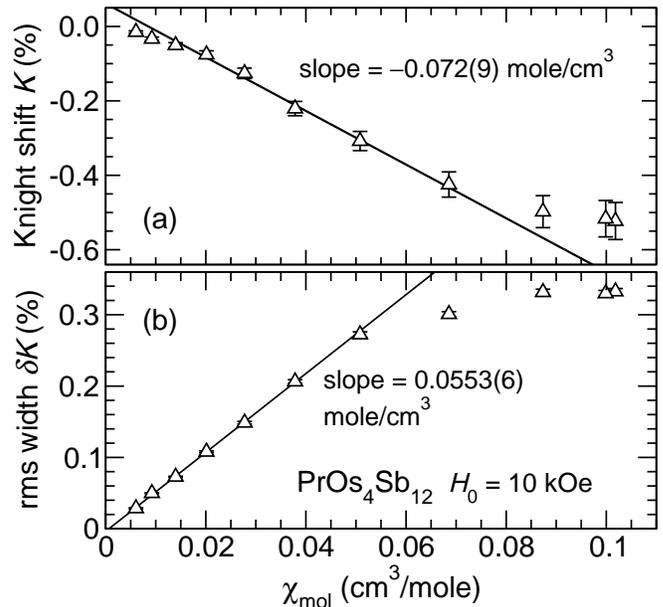
FIG. 5. (a) Clogston-Jaccarino plot of  $\mu^+$  Knight shift  $K$  vs molar susceptibility  $\chi_{\text{mol}}$  in  $\text{PrOs}_4\text{Sb}_{12}$ . Line: linear fit for  $\chi_{\text{mol}}$  in the range  $0.01\text{--}0.05\text{ cm}^3/\text{mole}$ . (b) rms width  $\delta K$  of Knight shift distribution vs  $\chi_{\text{mol}}$ . Lines: linear fits to points for  $\chi_{\text{mol}}$  between  $0.01$  and  $0.05\text{ cm}^3/\text{mole}$ .
