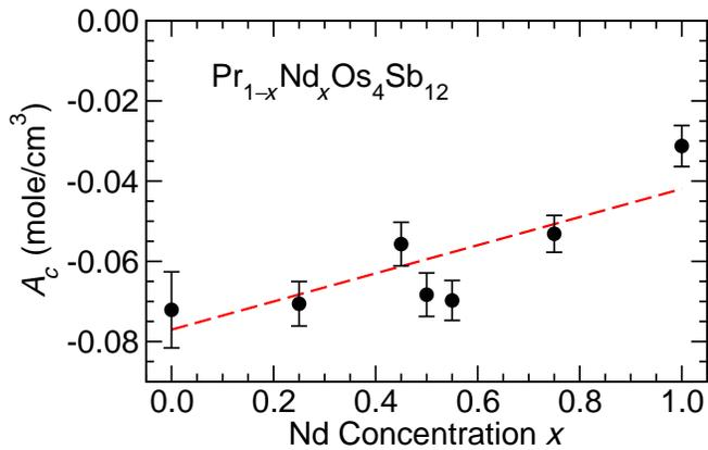
FIG. 8. (Color online) Dependence of initial Clogston-Jaccarino plot slopes  $A_c(x) = [dK(\chi, x)/d\chi]_0$  on Nd concentration  $x$  in  $\text{Pr}_{1-x}\text{Nd}_x\text{Os}_4\text{Sb}_{12}$ . Dashed curve: fit of Eq. (6) to the data.
