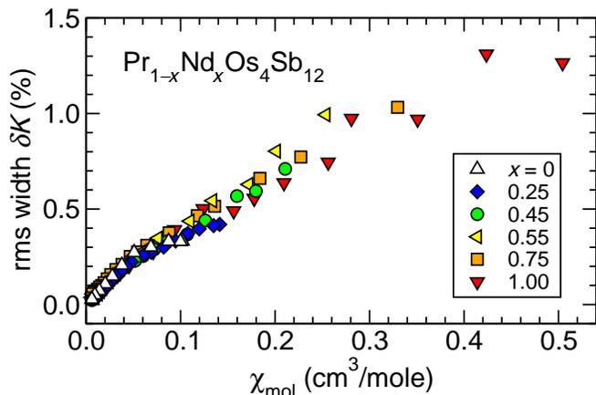
FIG. 7. (Color online) rms widths  $\delta K$  of Knight shift distribution vs  $\chi_{\text{mol}}$  for  $\text{Pr}_{1-x}\text{Nd}_x\text{Os}_4\text{Sb}_{12}$ , where  $x = 0, 0.25, 0.45, 0.55, 0.75,$  and  $1.00$ .
