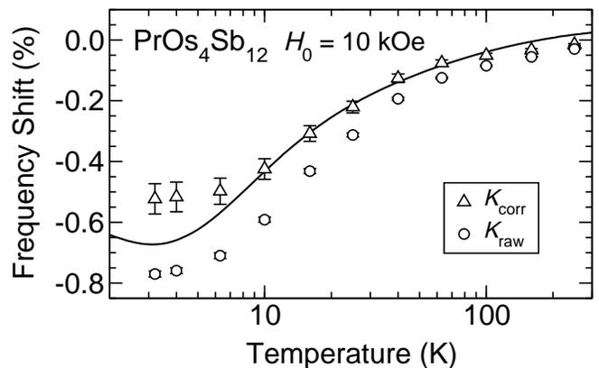
FIG. 3. Temperature dependence of fractional  $\mu^+$  frequency shifts in  $\text{PrOs}_4\text{Sb}_{12}$ .  $K_{\text{raw}}$ : raw shift.  $K_{\text{corr}}$ : Knight shift, corrected for Lorentz and demagnetization fields. Curve:  $K_{\text{lin}}(\%) = 0.06 - 7.2\chi_{\text{mol}}(T)$  (cm<sup>3</sup>/mole) (cf. Sec. III A).
