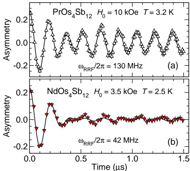
FIG. 2. (Color online)  $\mu^+$  time spectra displayed in rotating reference frames (rotation frequencies  $\omega_{\text{RRF}}$ ). (a)  $\text{PrOs}_4\text{Sb}_{12}$ , single-signal  $\mu\text{SR}$  spectrometer insert. (b)  $\text{NdOs}_4\text{Sb}_{12}$ ,  $\mu\text{SR}\times 2$  spectrometer insert, sample channel. Curves: fits to Eq. (1) to the data.
