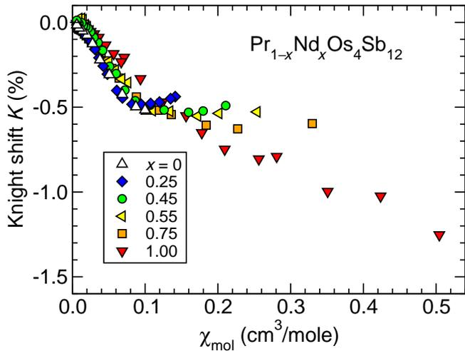
FIG. 6. (Color online) Clogston-Jaccarino plots of Knight shift  $K$  vs molar susceptibility  $\chi_{\text{mol}}$  for  $\text{Pr}_{1-x}\text{Nd}_x\text{Os}_4\text{Sb}_{12}$ , where  $x = 0, 0.25, 0.45, 0.55, 0.75,$  and  $1.00$ . For clarity the error bars are not shown.
