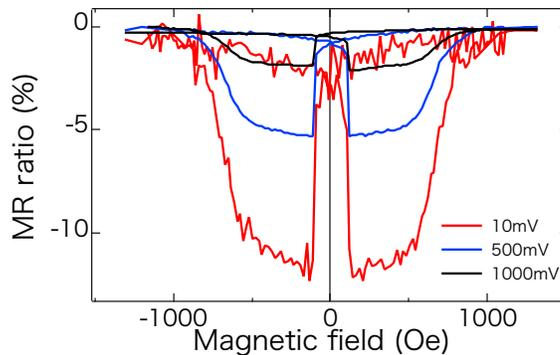
FIG. 3. TMR curve for MTJ of  $\text{MgO}(110)/\text{NiO}(110)$  (5 nm)/ $\text{Fe}_3\text{O}_4(110)$  (60 nm)/ $\text{Al}_2\text{O}_3$  (2.4 nm)/Fe (5 nm)/Co (10 nm)/Au (30 nm) at RT. Red, blue, and black lines are TMRs with bias voltages of 10, 500, and 1000 mV.
