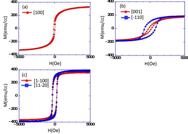
FIG. 2. Hysteresis curves obtained from VSM measurements at RT for epitaxial  $\text{Fe}_3\text{O}_4$  films with various crystal orientations. (a) is  $\text{Fe}_3\text{O}_4(100)$ , (b) is  $\text{Fe}_3\text{O}_4(110)$ , and (c) is  $\text{Fe}_3\text{O}_4(111)$ . Directions of magnetic fields are given in plots.
