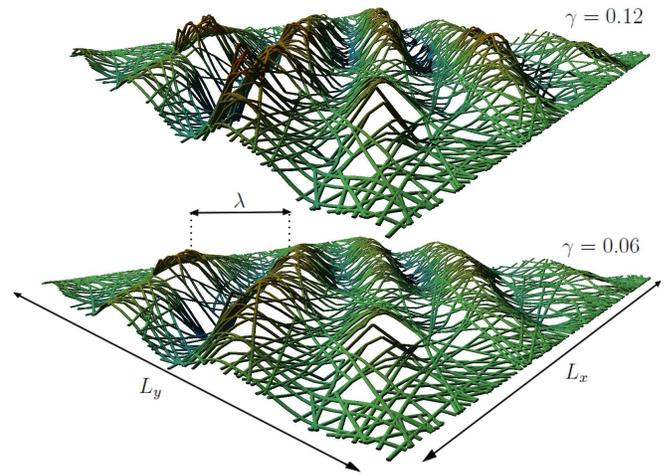
FIG. 1: Snapshots of a wrinkled random network ( $l_b/L = 2.5 \times 10^{-3}$  and  $\eta = 54$ ) at two different shear strains  $\gamma = 0.06$  and  $0.12$ . The dimensionless displacement  $z/\lambda$  in normal direction is color coded. Wrinkles form at an angle of 45° to the shearing direction; the wrinkle amplitude increases with the shear angle.
