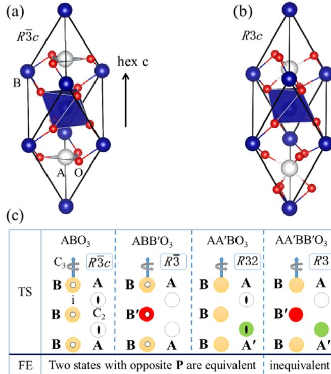
Figure 2. (a) and (b) show the paraelectric  $R\bar{3}c$  and ferroelectric  $R3c$  structures, respectively. The arrow indicates the hexagonal  $c$  axis. (c) illustrates how an asymmetric multiferroic can be designed by tuning the composition of the transition state (TS). The symmetry operations ( $C_3$ ,  $C_2$ ,  $i$ ) are denoted. Only in the case of  $AA'BB'O_6$ , the two locally stable FE states evolved from the TS are inequivalent.
