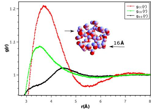
FIG. 1: Intermolecular partial pair distribution functions of supercritical CO<sub>2</sub>. Partial pair distribution functions and a heterogeneity generated by molecular dynamics simulations at T= 10000 K. The inserted heterogeneity, consist of carbon atoms (Red) and oxygen atoms (Silver Blue), was depicted from a simulated configuration.
