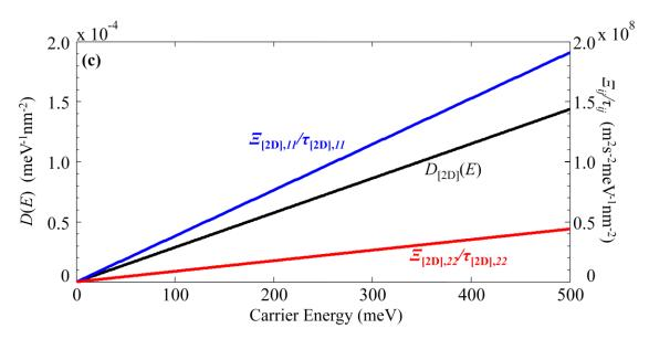
Fig. 3: Density of states and principal components of transport distribution tensor for twodimensional systems. (a) The parabolic conduction band valley at the *K* point of  $MoS_2^{20}$ . (b) The anisotropic Dirac cone in graphene supperlattice <sup>21, 22</sup>. (c) The anisotropic Dirac cone in bisectrix oriented Bi<sub>0.96</sub>Sb<sub>0.04</sub> thin films <sup>19, 23</sup>.
