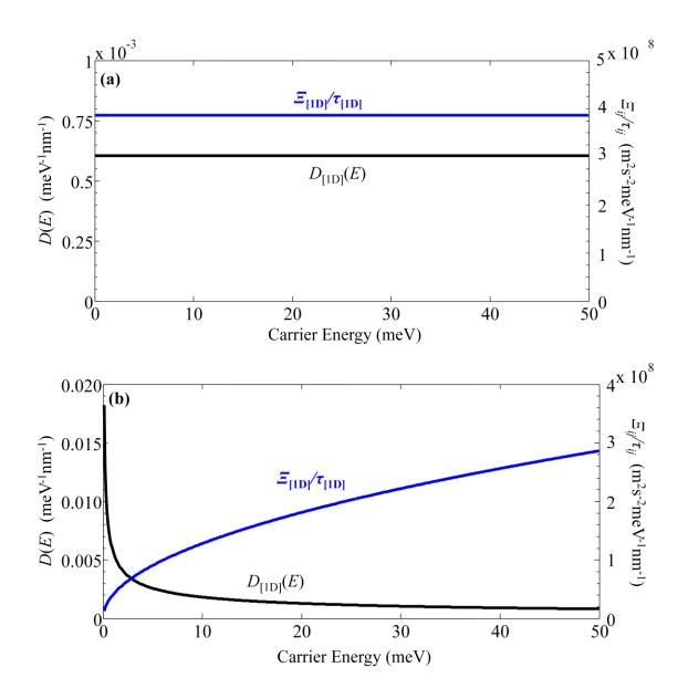
Fig. 4: Density of states and principal components of transport distribution tensor for onedimensional systems. (a) Metallic armchair carbon nanoribbon with a width of 6.02 nm and Dirac fermion group velocity of  $8 \times 10^5$  m/s<sup>24, 25</sup>. (b) Semiconducting armchair nanoribbon with a width of 21 nm, a band gap of 0.65 eV and an effective mass of  $0.05m_e^{24, 26}$ .
