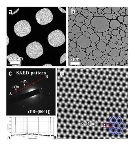
**Figure S2.** Characterization of high quality CVD graphene using HR-TEM and HAADF-STEM. a and b, TEM images of monolayer graphene on a Cu grid with amorphous carbon as support layer. c, Selected area electron diffraction (SAED) pattern of graphene monolayer, evidenced by the same intensity along the A-B line profile. d, Atomic resolution image of high quality graphene obtained by high-angle annular dark filed (HAADF) scanning transmission electron microscope (STEM).
