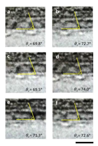
Figure S3. Cross-sectional TEM images of nanobubbles in a graphene liquid cell. a-f, TEM images showing the contact angles of nanobubbles in water trapped between sandwiched graphene, ranging from 70 to  $74^{\circ}$  (see supplementary Movie S1). The average contact angle of the nanobubbles is  $\sim 72^{\circ}$ . Scale bar, 5 nm.
