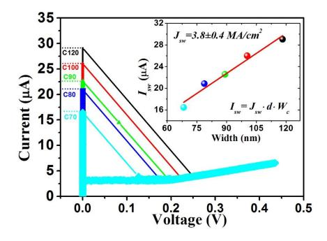
FIG. 2. I–V curves of five single nanowires (120 nm wide and 20  $\mu$ m long) with constrictions of different widths. I–V curves from top to bottom correspond to the width of the constrictions of 120 (i.e., no constriction), 100, 90, 80, and 70 nm, respectively. The inset shows the relationship between  $I_{sw}$  and  $W_c$ . The red line indicates the linear fitting equation  $I_{sw} = J_{sw} \cdot d \cdot W_c$ , where d=6.5 nm is the thickness of the nanowire.
