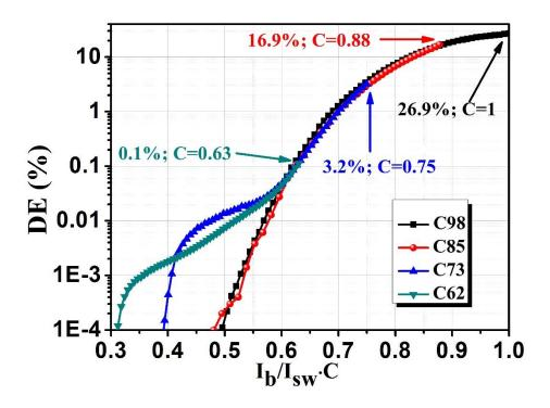
FIG. 4. DE of devices with different constriction sizes versus the normalized biased current. The values of C and the maximal DE are indicated. The lines are provided as a guide to the eye.
