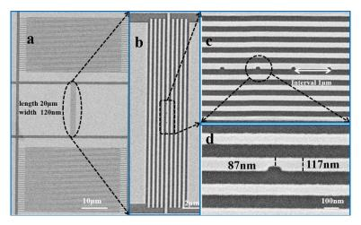
FIG. 1. SEM images of a single nanowire sample. (a) Full SEM image of a single nanowire with two long, wide meandering nanowires in series and 8 neighboring nanowires in parallel. (b) Zoom-in of the single nanowire with 8 neighboring nanowires in parallel. (c) Zoom-in of the nanowire, including four artificial constrictions at 1 µm intervals. (d) Zoom-in of one artificial geometric constriction. The dimension of the constriction and the nanowire is consistent with the design.
