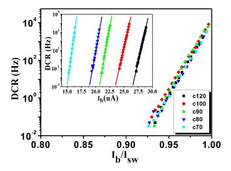
FIG. 3. DCR as a function of the bias current normalized by the switching current. The inset shows the DCR of the SNSPDs with different constriction widths as a function of the bias current. The straight lines in the inset are provided as a guide to the eye.
