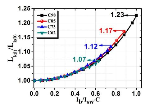
FIG. 5. Current dependence of the normalized kinetic inductance.  $L_k(0)$  represents the inductance of SNSPDs at 2.3 K without the current bias. The lines in the inset are provided as a guide to the eye.
