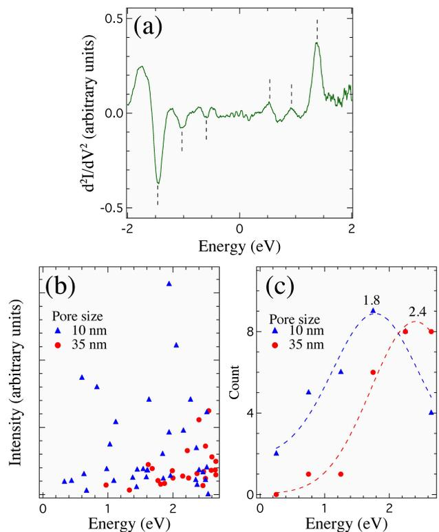
FIG. 2. (Color online). (a) Typical  $d^2I/dV^2$  curve from a NPG film. Dashed lines are guides to the eye. (b) Energy and intensity distributions of the plasmon peaks in the  $d^2I/dV^2$  curves for NPG films of 10 nm (blue) and 35 nm (red) pores. (c) Gaussian distributions (dashed lines) of the plasmon peaks in (c).
