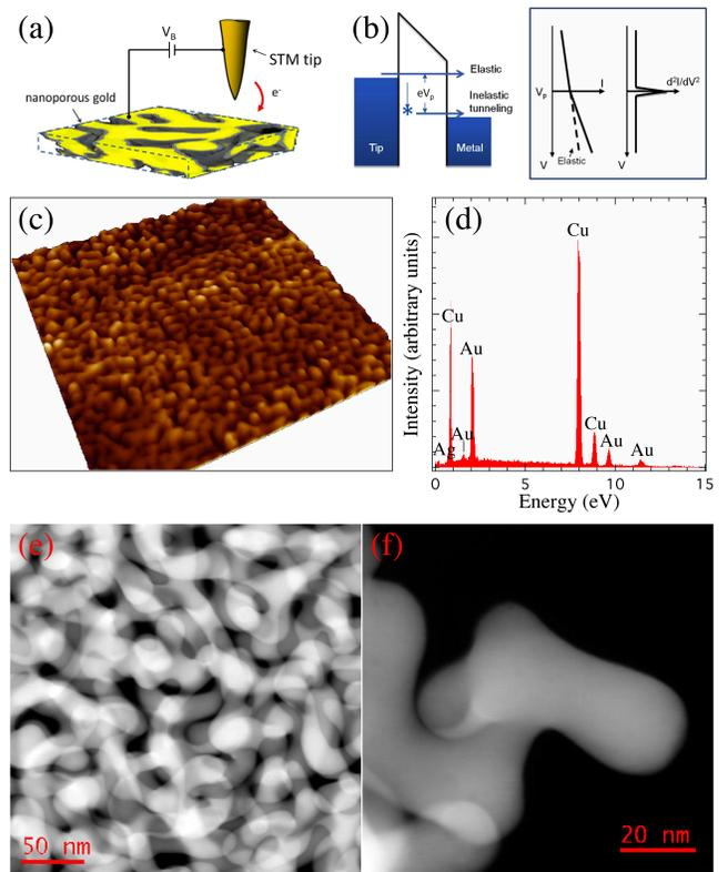
FIG. 1. (Color online). (a) Schematic representation of inelastic tunneling microscopy from a NPG film in a STM. (b) Illustration of inelastic tunneling spectroscopy. (c) A typical STM topographic image of a NPG film. The scan size is  $2 \times 2 \mu\text{m}^2$ .  $V_B = -1.0 \text{ V}$ ,  $I_t = 1.0 \text{ nA}$ . (d) EDX spectrum of a dealloyed NPG film. STEM images of non-annealed NPG film containing  $\sim 5 \text{ at. \%}$  residual Ag in (e) and detailed image in (f).
