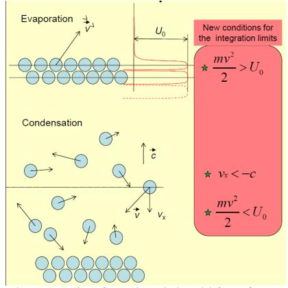
Figure 1. Schematic representation of new theoretical model for surface evaporation and recondensation onto the surface.
