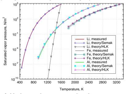
Figure 2. Metal saturated vapor pressure dependence on temperature: comparison of the new theory ("Semak") with simplified Hertz-Langmuir-Knudesen/Clausius-Clapeyron equation ("HLK") and experimental data ("measured").
