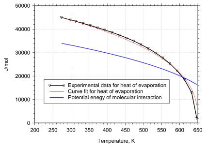
Figure 3. Experimentally measured specific latent heat of evaporation of water,  $L_v$ , (note it drops to zero at the critical temperature) and the product of temperature dependent depth of potential barrier,  $U_0$ , and the Avogadro number (in order to express potential well depth in units of J/mol).
