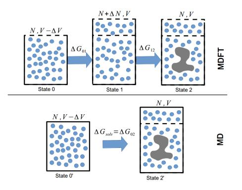
Figure 1: Thermodynamic scheme for the computation of the solvation free energy using the MDFT in the grand-canonical ensemble (top) or the molecular dynamics free energy perturbation method in the isobaric-isotherm ensemble (bottom). In the thermodynamic limit, states 0 and 0' and states 2 and 2' are equivalent, which motivates eqs. (11) and (16) in the text.
