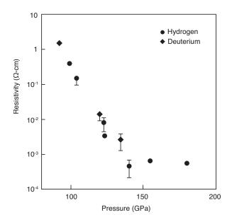
Fig.8. Electrical resistivity of fluid H versus multiple-shock pressure [4]. Corresponding temperatures are 1500 to 3000 K. Density at end of crossover from fluid semiconductor to fluid metal is 0.32 mol  $H_2/cm^3=0.64$  mol  $H/cm^3$ . Free-electron Fermi temperature  $T_F$  at this density is  $T_F=220,000$  K. Metallic fluid H is degenerate  $(T/T_F \approx 0.014)$ . Wigner and Huntington predicted their IMT from insulating  $H_2$  to metallic H at 0.62 mol H/cm<sup>3</sup>[1].
