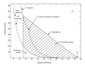
Fig. 4. Hugoniot, isentrope, and 0-K isotherm of liquid Ar plotted as pressure versus molar volume [30].
