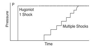
Fig. 2. Schematics of applied pressure histories of single-shock and multiple-shock compressions. Both compressions are adiabatic. However, multiple-shock compression is quasi-isentropic, as well. Dissipation T and S are induced in rapid step increases, while during times of nearly constant pressure compressions are essentially isentropic. By pulse shaping multiple-shock wave, T and S are reduced substantially from those caused by single sharp jump to same pressure.
