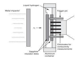
Fig. 6. Dynamic compression experiment on liquid  $H_2$  initially at 20 K. Liquid  $H_2$  diameter and thickness were 28 mm and 0.5 mm, respectively.
