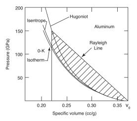
Fig. 3. Hugoniot, isentrope, and 0-K isotherm of Al [29], as well as Rayleigh line, plotted as pressure versus specific volume.  $V_0$  is crystal volume at ambient. Isentrope and isotherm are reversible; Hugoniot is not. Irreversible thermal-dissipation energy of Hugoniot is represented by cross-hatched area.
