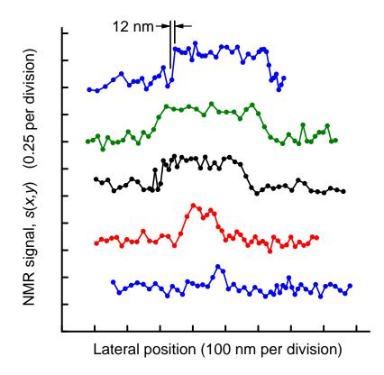
**Figure 3 – Line scans showing the NMR signal as a function of position.** A stepwise increase in NMR signal is seen when the sample is positioned over the NV center. The step height corresponds to a proton field of approximately  $(300 \text{ nT})^2$ . Spatial resolution is about 12 nm, limited primarily by the scan step size and scan position irregularities. For clarity, successive scans are displaced vertically by two divisions.
