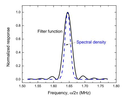
**Figure S1** – Normalized plots of the filter function and proton magnetic field spectral density. Filter function assumes N = 96 and  $\tau = 304$  ns. Filter bandpass is 30 kHz FWHM. The magnetic field spectral density is assumed to have a Gaussian line shape centered at 1.64 MHz with FWHM of 20 kHz.
