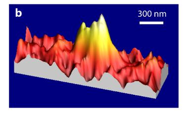
**Figure 4 – Two dimensional NMR images.** Results are from two different PMMA samples with two different NV centers. Height shown is proportional to s(x,y). Apparent roughness is primarily due to photon shot noise. The image in (a) incorporates the line scan data shown in Fig. 3.
