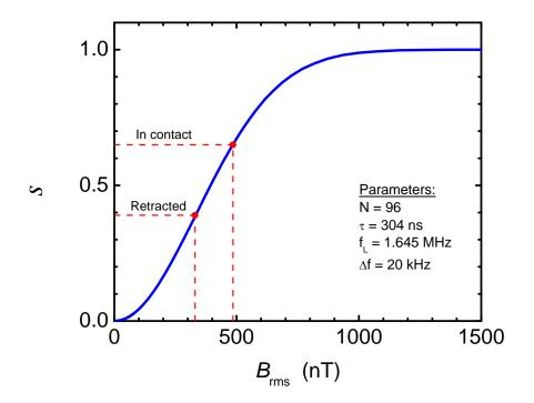
**Figure S2** – NV signal response *s* as a function of the rms amplitude of the magnetic field. Signal values and associated proton magnetic fields for the coherence dips in Fig. 2 (main text) are indicated.
