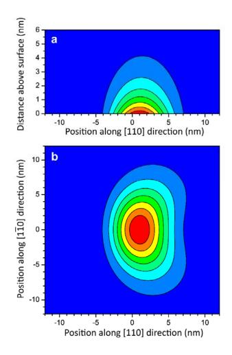
**Figure 5 – Calculated point spread function for a 10 nm deep NV.** (a) Vertical cross-section of the response shows that the signal falls by one-half for protons located 1.3 nm above the diamond surface. The maximum response is slightly shifted laterally with respect to the NV position due to the [111] orientation of the NV axis. (b) Lateral response at the diamond surface is shown. The PSF width is slightly asymmetrical, with the narrowest being 6 nm FWHM in the [110] direction.
