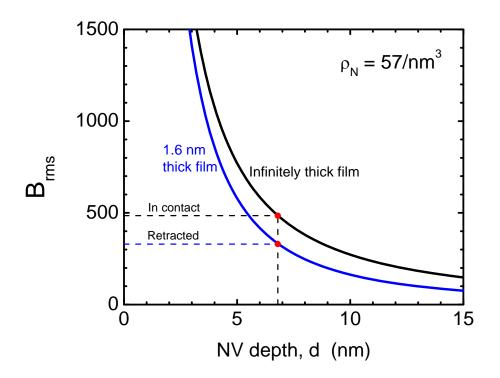
**Figure S3** – Theorectical magnetic field at the NV center from protons on the diamond surface as a function of NV depth. The two field values corresponding to the coherence dips in Fig. 2 (main text) are indicated.
