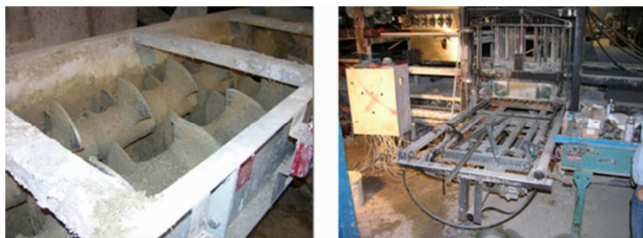
Figure 2. Precasting method (left : mixer, right : block press)
