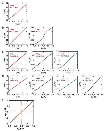
**Figure S2. a-d**, Contact I-V curves between each tip and the single-layer FeSe film measured by the -µm-probe-separation 4PP at 90 K when one (**a**), two (**b**), three (**c**) and four (**d**) tips have touched the FeSe film. **e**, The 4PP I-V curve showing non-superconducting behavior measured after the contact I-V measurement of **d**.
