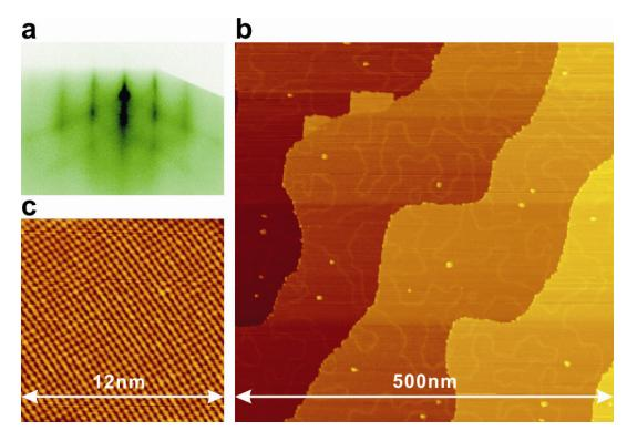
Figure 1. Growth and characterization of high-quality single-layer film of FeSe. a, RHEED pattern taken just after the growth of the film. b,c, Large- and atomic-resolved STM images of the film, taken at 7 K with  $V_s$ = 3.00 V and  $I_t$ = 100 pA and at 3 K with  $V_s$ = 0.05 V and  $I_t$ = 250 pA, respectively.
