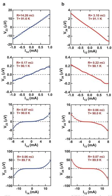
**Figure S3.** 4PP transport measurement on Bi2212 crystal with measurement configurations of C1423 (a) and C1234 (b), respectively. The sample temperatures and linearly fitted resistance around zero current are shown in each figure.
