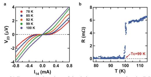
**Figure S4.** Temperature dependence of electrical transport property of another FeSe/STO sample measured with the 100- $\mu$ m-tip-separation 4PP fixed at one measuring location while temperature was increasing. **a**, Typical I-V curves taken at various temperatures. **b**, Temperature dependence of the resistance obtained from a linear fit to the I-V curves. A critical temperature of 99 K was observed.
