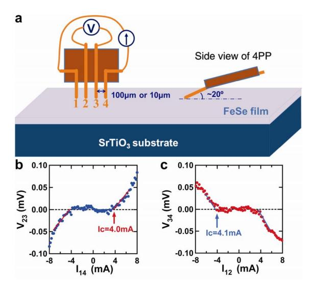
**Figure 2. a**, Schematic of 4PP transport measurement setup. The numbers are used to denote the contacting tips. All four tips can touch the sample surface gently in an inclined angle of ~20°. **b**,**c**, Typical superconducting I-V curves taken with a tip separation of 10  $\mu$ m at 3.0 K with measurement configurations of C1423 and C1234, respectively.
