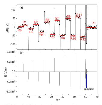
FIG. 3. Electric field induced switching between multiple memory states (a) with a corresponding electric field time profile (b).
