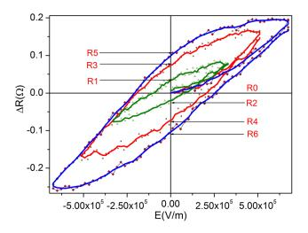
FIG. 2. Electroresistive hysteresis of CoFe film with multi memory states. Solid lines represent smoothed experimental results.
