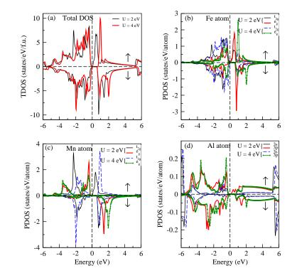
**Figure 8.** (Color online) Total and partial density of states plots for  $Fe_2MnAl$  in the ferromagnetic phase in the presence of U. Shown are (a) the TDOS plot, (b) PDOS of Fe atom, (c) PDOS of Mn atom and (d) PDOS of Al atom.
