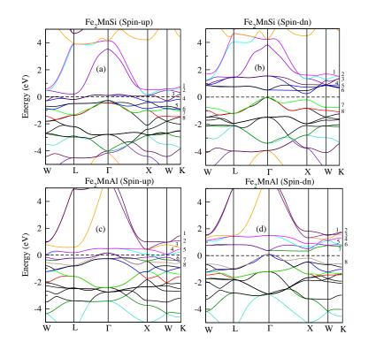
**Figure 4.** (Color online) Electronic band structures in the ferromagnetic phase (a and b) for spin-up and spin-dn channels of Fe<sub>2</sub>MnSi and (c and d) for spin-up and spin-dn channels of Fe<sub>2</sub>MnAl.
