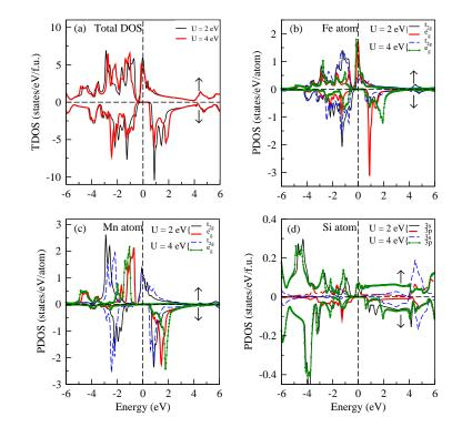
**Figure 7.** (Color online) Total and partial density of states plots for  $Fe_2MnSi$  in the ferromagnetic phase in the presence of U. Shown are (a) the TDOS plot, (b) PDOS of Fe atom, (c) PDOS of Mn atom and (d) PDOS of Si atom.
