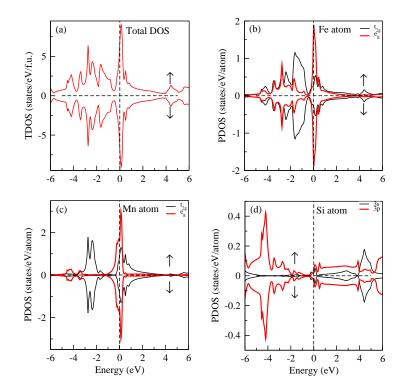
Figure 2. (Color online) Total and partial density of states plots for  $Fe_2MnSi$  in the paramagnetic phase. Shown are (a) the TDOS plot, (b) PDOS of Fe atom, (c) PDOS of Mn atom and (d) PDOS of Si atom.
