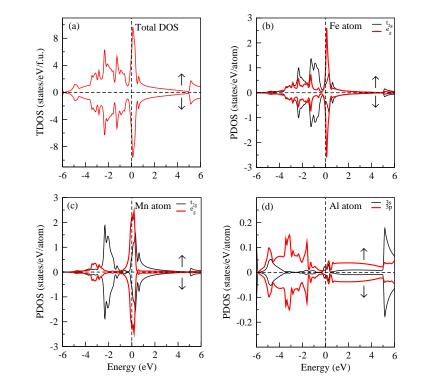
Figure 3. (Color online) Total and partial density of states plots for  $Fe_2MnAl$  in the paramagnetic phase. Shown are (a) the TDOS plot, (b) PDOS of Fe atom, (c) PDOS of Mn atom and (d) PDOS of Al atom.
