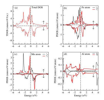
Figure 6. (Color online) Total and partial density of states plots for  $Fe_2MnAl$  in the ferromagnetic phase. Shown are (a) the TDOS plot, (b) PDOS of Fe atom, (c) PDOS of Mn atom and (d) PDOS of Al atom.
