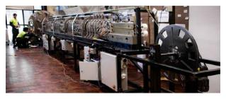
Figure 7. Device for assembling 15/5 (15 strands with 5 mm width) Roebel cables (courtesy IRL-General Cable).
