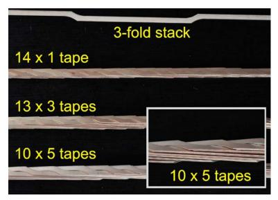
Figure 8. Multi-stacking of strands: a 3-fold stack of punched CC tapes and 3 different Roebel cables with 4 mm width are shown. The upper cable consists of 14 single tapes, whereas the middle and the lower cables consist of 13 3-fold stacks and 10 5-fold stacks, respectively.
