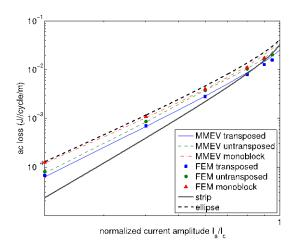
Figure 20. Transport AC loss for transposed and untransposed strands with a cross-section representative of that of a Roebel cable (two stacks of tapes), calculated using two different models (FEM and MMEV, refer also to Figure 18) and compared to the loss of a rectangular monoblock. Figure reprinted from [67].
