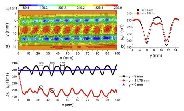
Figure 14. Exemplary magnetic field map obtained by Hall probe scanning technique. The field profiles along different lines in the x- and y- direction are also plotted. The applied field is 230 mT. Note the different scales adopted for the width and the length of the cable in a), which make the aspect ratio of the cable different from the real one. Reprinted from [32].
