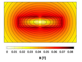
Figure 13. FEM-calculated self field pattern in the cross section of a Roebel cable. Each tape represents the different positions assumed by a tape along one transposition length. Redrawn from [47].
