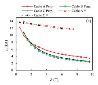
Figure 12. Field dependence of the critical current for different cable samples at 4.2 K. Cable A is from GCS, cables B and C from KIT. Source: [44].
