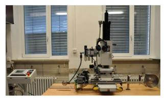
Figure 5. Reel-to-reel computer controlled pneumatic punching machine utilized at KIT for producing Roebel strands. The mechanical punching tools can be changed for obtaining cable widths between 4 and 12 mm. At present the transposition length for 4 mm-wide tape is 115.7 mm, whereas for 12 mm-wide tape it is 126 mm.
