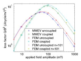
Figure 18. Comparison of the magnetization loss in a 14-strand Roebel cable for the cases of full coupling and full uncoupling between the strands, calculated with the power-law and critical state models, solved with finite element (FEM) and Minimum Magnetic Energy Variation methods (MMEV). Reprinted from [67].
