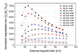
Figure 21. Reduction of magnetization loss due to Roebel cabling (S0\_N10) and successive filamentarization (S5\_N10) with respect to the loss in the original coated conductor (S0\_N1). The angles represent the orientation of the magnetic field with respect to the flat face of the cable. Reprinted from [30].
