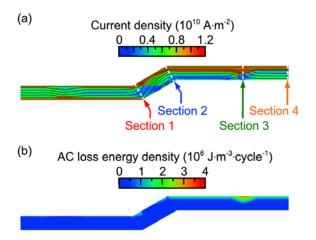
Figure 19. Current density (a) and AC loss density (b) distributions in a six-strand Roebel cable carrying AC current and subjected to an AC perpendicular magnetic field. Reprinted from [75].
