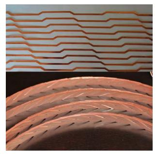
Figure 6. Ten strands punched from 12 mm-wide coated conductor, before (top) and after (bottom) they are assembled into cable.
