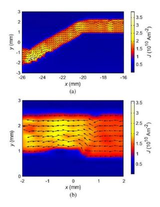
Figure 15. Two examples of current flow (reconstructed from Hall probe scan measurements) close to local defects: (a) a defect at the inner left corner leads to an enhancement of the current density close to the opposite edge (yellow – compare with the right corner, which does not present such defect); (b) due to a reduction of the cross section, the current density is increased in the left section. Reprinted from [48].
