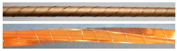
Figure 10. Pictures of two cable designs alternative to the Roebel: Top: Cable on Round Core (CORC), source: [40].; b) Twisted Stacked Tape Cable (TSTC), source: [41]. The thin wire around the CORC sample is for mechanical support during the twisting process.
