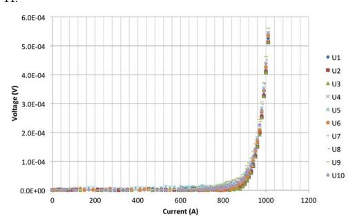
Figure 11. Current-voltage characteristics for the Roebel cable used in [42,43], measured on the 10 different composing strands. The critical current corresponding to the 1  $\mu$ V/cm criterion (450  $\mu$ V for a distance between the voltage taps of 4.5 m) is about 1 kA. The value of 936 A used in the references and in the table of section 3.6 refers to a lower critical voltage.
