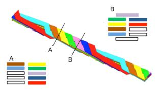
Figure 3. Schematic illustration of a Roebel bar made from coated conductor tapes. Two transversal cross-sections at different positions are also shown.
