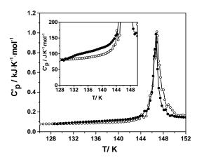
**Figure 6.** Comparison of the FSC thermograms of a toluene film vapor-deposited at 112 K with that of a film which was vapor deposited at 112 K and then heated with a rate of 0.5 K/s to 128 K. The decrease in the width of the endotherm and the increase in the heat capacity at temperatures below the onset of the FREs are consistent with partial transformation of the stable film into ordinary supercooled liquid during slow heating. See text for discussion.
