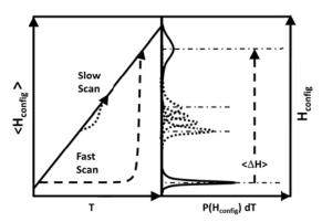
**Figure 7.** Illustration of fundamental difference between FSC and traditional DSC. Due to high heating rates fast relaxation in FSC experiments takes place at temperatures which are significantly higher than the starting temperature of the scan. As argued in the text, this leads to a significant separation between the enthalpy distribution of the initial (stable vapor-deposited glass) and final (ordinary liquid), which greatly simplifies kinetics of the relaxation in the case of rapid scans.
