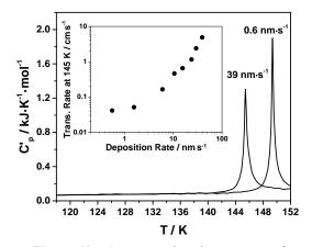
**Figure 10.** Representative thermograms of stable toluene films vapor deposited at distinct rates at 112 K. Inset shows the absolute transformation rate values at temperature of 145 K during the transformation for the films prepared at eight distinct deposition rates. The rate is reported in the transformation front velocity units (cm/s). See Fig. 11 and text for discussion.
