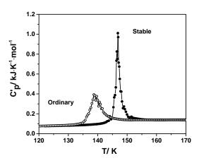
**Figure 5.** Comparison of fast relaxation endotherms of the most stable vapordeposited toluene film with that of an ordinary glass prepared by slow cooling of melt from 127 to 112 K. The onset temperature of FRE of vapor deposited sample is 10 K higher than that of the ordinary glass which signifies a greater kinetic stability of the vapor-deposited film
