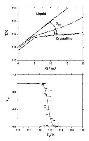
**Figure 3.** *Upper panel:* Heating curves of micrometer scale isobutane vapor deposited at temperatures above and below its melting point. The deposition temperature (as read by DAQ system) is inferred by extrapolating the heating curve to zero heat. The changing slope of the heating curves signifies the extent of sample crystallinity (see text for details).
