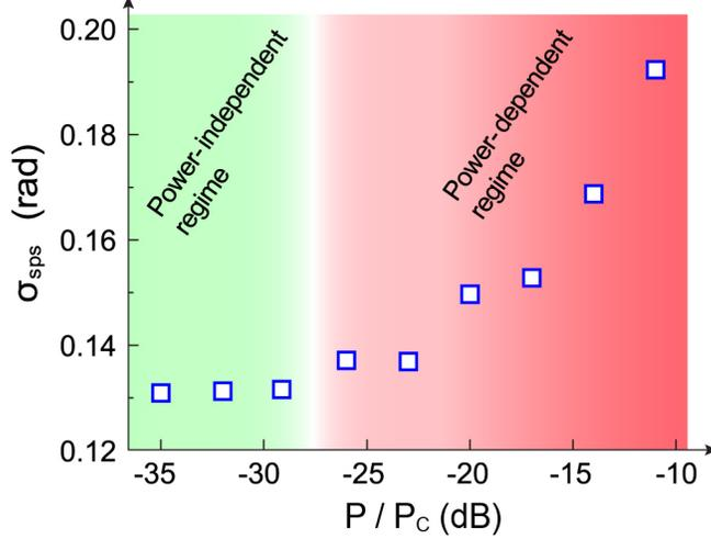
FIG. 4. Dependence of the standard deviation of SPS switching current distribution on the reduced input power of the microwave signal. The measurements are made at 60 mK.  $P_c$  corresponds to a power that induces in the wires a current equal to their critical current.
