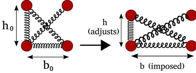
FIG. 2: Minimal rectangular model consisting of one  $x$ -oriented, one  $y$ -oriented, and two diagonal springs.  $b_0$  and  $h_0$  are the base and height of the rectangular cell in the unstrained state. Under strain,  $b_0 \rightarrow b$  and the height is free to adjust in order to minimize the elastic energy,  $h_0 \rightarrow h$ .
