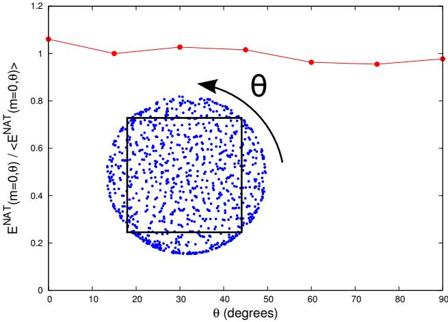
FIG. 10: Zero-field elastic modulus  $E^{\text{NAT}}(m = 0)$  calculated with NAT for the experimental lattice drawn in the inset picture varying the rotation angle  $\theta$ . To illustrate the effective isotropy we plot the elastic modulus rescaled by the average of  $E^{\text{NAT}}(m = 0)$  over  $\theta$ . The black square in the inset contains the block of particles extracted from the experimental data after the rotation and used in our calculation.
