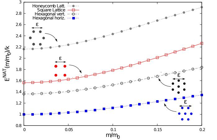
FIG. 7: Elastic modulus  $E(m/m_0)/k$  calculated with NAT for  $\mathbf{m} \parallel \hat{z}$  for the different lattices shown. We indicate the direction of the applied strain by  $\varepsilon$ . The magnetic interaction is purely repulsive and strengthens the elastic modulus in this configuration.
