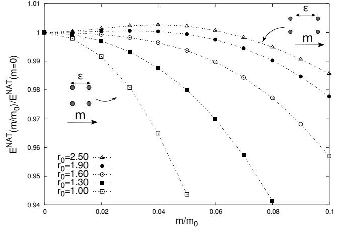
FIG. 5: Rectangular lattice with  $\mathbf{m} \parallel \hat{x}$ . Different trends of  $E^{\text{NAT}}(m/m_0)$  are shown for different unstrained lattice shapes using the undeformed base-height ratio  $r_0$  as shape parameter. We indicate the direction of the applied strain by  $\varepsilon$ . To compare and enhance the different trends,  $E^{\text{NAT}}(m/m_0)$  is rescaled by  $E^{\text{NAT}}(m = 0)$ .
