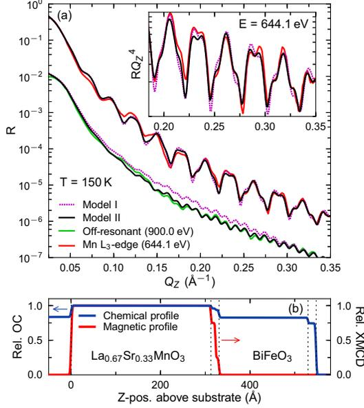
FIG. 4. (color online) a) X-ray reflectivity data measured at 644.1 eV and 900.0 eV, i.e. resonant at the Mn  $L_3$  edge and off-resonant. The data was fitted using two different models as described in the text. The inset shows  $RQ_z^4$  in the most sensitive high  $Q_z$  region. b) Resulting chemical (through XRR) and magnetic (PNR and XRMR) depth profiles.
