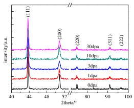
Fig. 2a. (color online)The normalized GIXRD patterns of Ni-17Mo-7Cr alloy specimens irradiated with 3MeV Au ions: from bottom to top, the dpa number is 0,1,3,10,30, respectively
