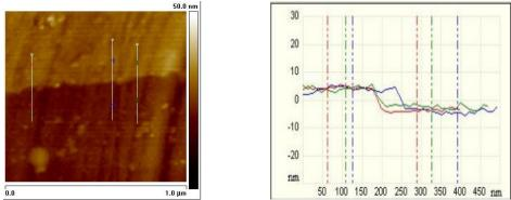
Fig. 3.(color online)(a) The AFM image of the irradiated and unirradiated zone of the Ni-17Mo-7Cr alloy specimen;(b) The measured step height
