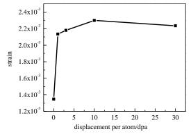
Fig. 2b. Microstrain of Ni-17Mo-7Cr alloy specimens irradiated at different dpa.
