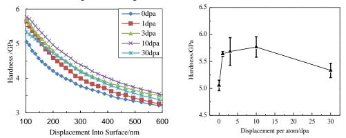
Fig. 4. (color online)(a)The near surface hardness as a function of contact depth, as measured by the nanoindenter; (b)The hardness of the specimens as a function of dpa at 100nm contact depth
