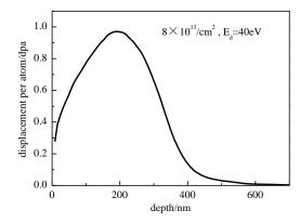
Fig. 1. SRIM 2006 calculation of the damage profile produced by 3MeV Au ion irradiation in Ni-17Mo-7Cr alloy
