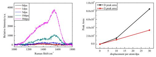
Fig. 5. (color online) (a)Raman spectra of the Ni-17Mo-7Cr alloy specimens irradiated at different ion fluences; (b) Areas of D and G peaks at different dpa.
