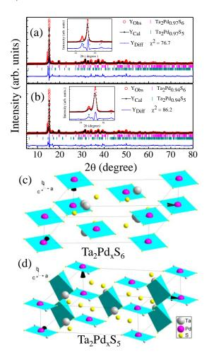
Figure 1 (Color online). Rietveld refinement for powder XRD patterns of compounds (a)  $Ta_2Pd_{0.97}S_6$  and (b)  $Ta_2Pd_{0.94}S_6$  with monoclinic space group C2/m. The XRD patterns are refined simultaneously for the two different crystal structures (c)  $Ta_2Pd_xS_6$  (magenta bars) and (d)  $Ta_2Pd_xS_5$  (cyan bars), respectively.
