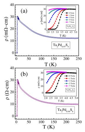
**Figure 2** (Color online). Temperature (T) dependences of resistivity ( $\rho$ ) for compounds (a) Ta<sub>2</sub>Pd<sub>0.97</sub>S<sub>6</sub> and (b) Ta<sub>2</sub>Pd<sub>0.94</sub>S<sub>6</sub>, whereas insets show  $\rho$  verses T at different applied magnetic fields upto 7 Tesla, respectively.
