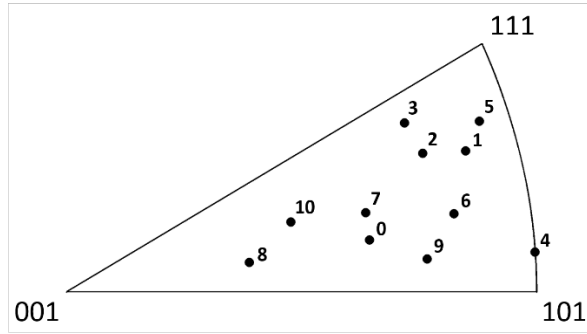
Figure 6. Stereographic triangle showing the random evolution of the misorientation axis for a single rotating grain as a function of cycle number.
