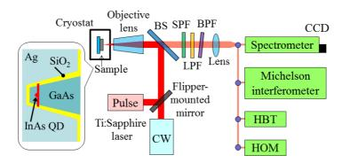
FIG. 1. Schematic of the measurement setup.
