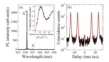
FIG 6. (a) PL spectrum measured under the quasi-resonant excitation. The inset shows the Rabi oscillation of the  $X^0$  emission intensity. (b) Semi-log plot of the measured second-order intensity correlation of the  $X^0$  emission under the  $\pi$ -pulse excitation. The red curve is the theoretical fit to the data.<sup>36</sup>
