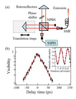
FIG. 3. (a) Experimental setup of Michelson interferometer for measuring the coherence time. NPBS: non-polarizing beam splitter. The phase shifter was introduced to record the interference fringes at a fixed optical-path length difference set by the translation stage. (b) The visibility as a function of delay time for the  $X^-$  emission. The inset shows an example of interference fringes at a position close to zero time delay.
