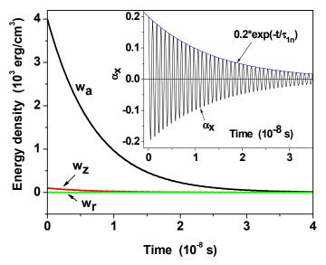
Fig. 1 The time dependence of the particular energies of magnetic nanoparticle for the high-frequency mode  $v_1$  which corresponds to the usual ferromagnetic resonance. Inset shows the behavior of the  $\alpha_x$  component of the unit magnetization vector.
