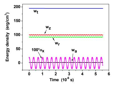
Fig. 2. The particular energies of magnetic nanoparticle for the low-frequency mode  $v_2$ . Note the enlarged scale of the time axis as compared with Fig. 1. The dotted line shows the  $\alpha_x$  component increased by a factor 100.
