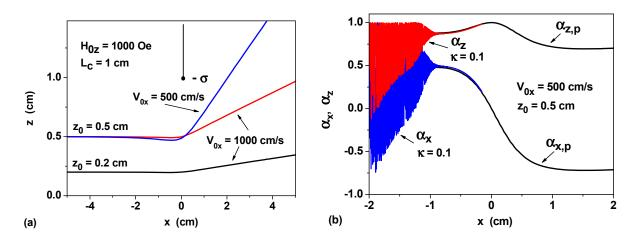
Fig. 5. a) The trajectories of a passive magnetic moment at different initial velocities  $V_{0x}$  and impact parameters  $z_0$ ; b)  $\alpha_x$  and  $\alpha_z$  components of the unit magnetization vector of magnetic nanoparticle as functions of the *x* - coordinate in comparison with the corresponding components  $\alpha_{x,p}$  and  $\alpha_{z,p}$  of the passive magnetic moment. The initial parameters of the particle and passive moment are the same,  $V_{0x} = 500$  cm/s,  $z_0 = 0.5$  cm.
