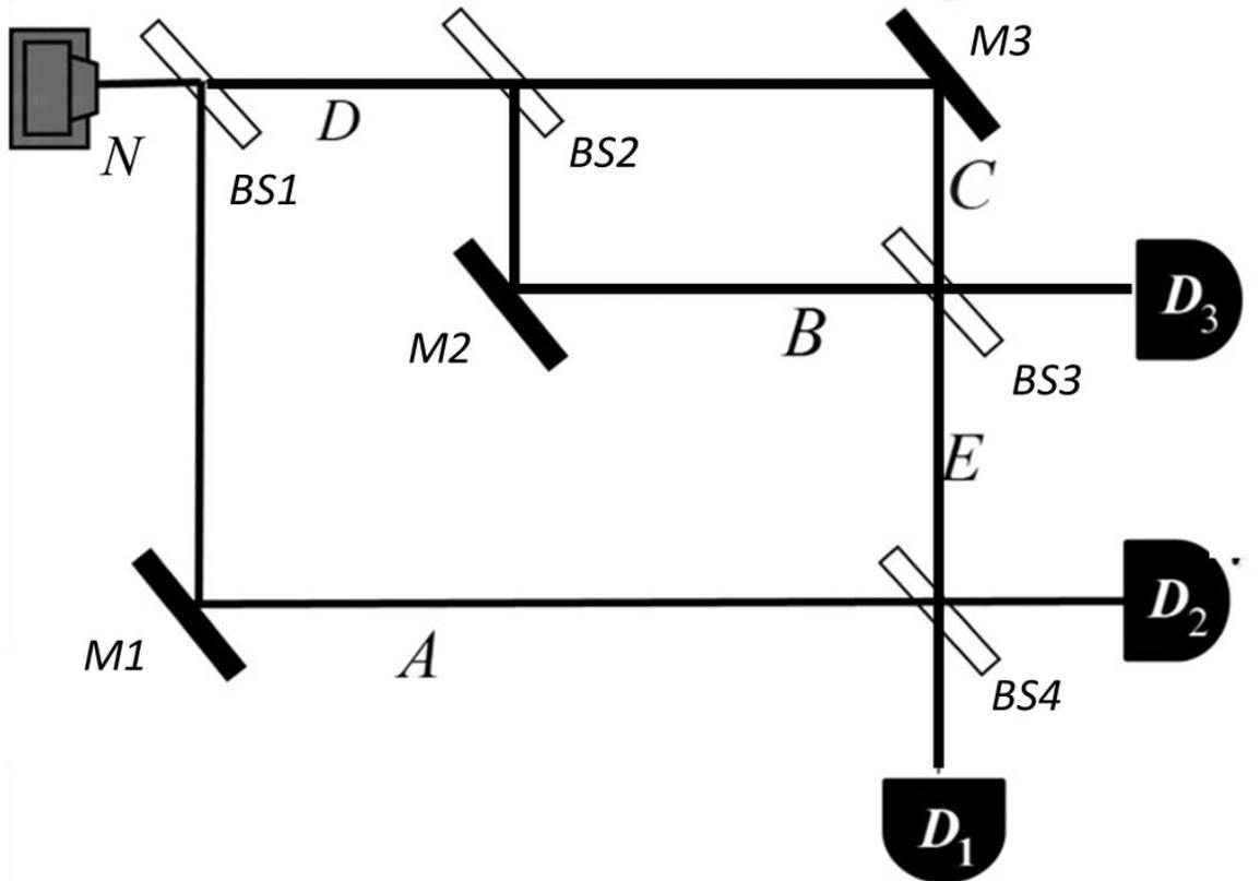
FIG.1. The nested Mach-Zehnder interferometer setup. The arm directing the photons from the photon source into the set-up is denoted  $N$ . Symbols  $A$  through  $E$  denote the interferometer arms,  $BS1$  to  $BS4$  are beamsplitters,  $M1$  to  $M3$  are mirrors, and  $D_1$  to  $D_3$  are detectors. (Adapted from Vaidman [1])
