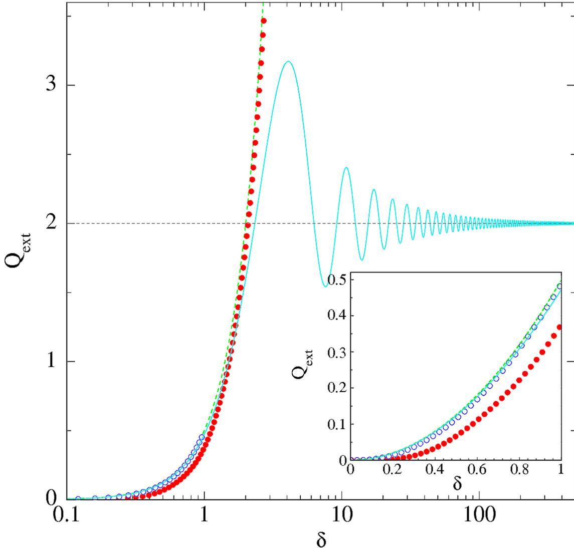
FIG. 1: Comparison between of the efficiency factor  $Q_{ext}^0$  obtained from Eq. (59) (full line), and the 2nd order approximation in  $\Delta n_p$  from Eq. (51, for  $\Delta n_p = 0.05$  (open dots) and  $\Delta n_p = 0.2$  (full dots). The broken line shows the Rayleigh–Gans approximation  $Q_{ext}^0 = \delta^2/2$ . The region with  $\delta \leq 1$  is expanded in the inset.
