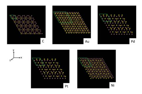
**Figure S1**: Relaxed atomic structures for the 5 different contacts considered. The green boxes denote the unit cell.
