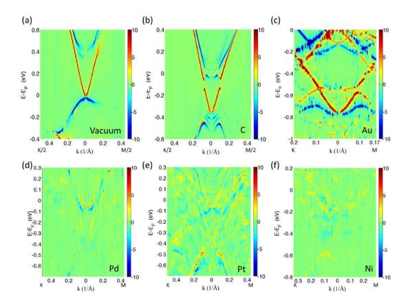
**Figure 5.** Spectral function (in units of 1/eV) projected on the first quintuplet and filtered for spin-momentum locking in the case of (a) vacuum, (b) graphene, (c) Au, (d) Pd, (e) Pt, and (f) Ni.
