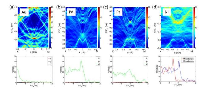
**Figure 4.** The top panels show the spectral function (in units of 1/eV) projected on the first Bi<sub>2</sub>Se<sub>3</sub> quintuplet when in contact with different metals, and the bottom panels are the density of states of isolated metal slabs with the same normalization used in all 4 cases.
