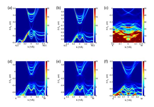
**Figure S3**: Bandstructure projected on the second quintuplet for the 6 cases considered: (a) vacuum, (b) graphene, (c) Au, (d) Pd, (e) Pt, and (f) Ni.
