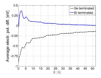
**Figure S2**: Band-bending in the  $Bi_2Se_3$  for Pd contacts when the surface termination is artificially changed from Se to Bi (the average metal-TI separation is the same in both cases).
