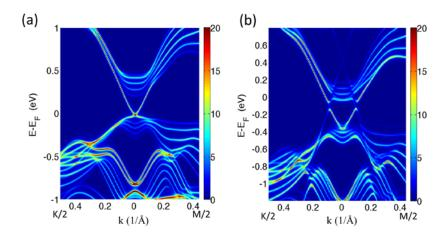
**Figure 3.** (a) Spectral function (in units of 1/eV) projected on the first Bi<sub>2</sub>Se<sub>3</sub> quintuplet when in contact with vacuum. (b) Spectral function projected on the first Bi<sub>2</sub>Se<sub>3</sub> quintuplet when in contact with graphene.
