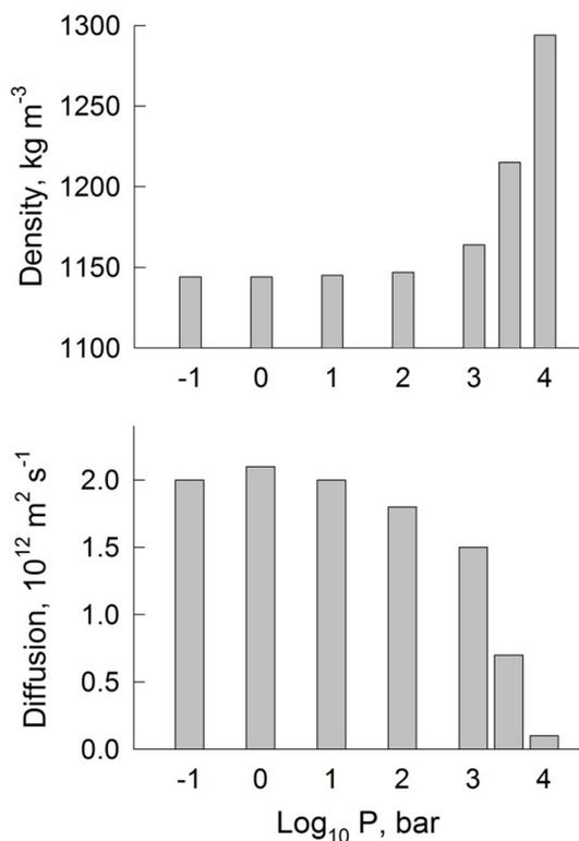
**Figure 7.** (Top panel) density of bulk [C<sub>2</sub>C<sub>1</sub>IM][Cl] vs. external pressure; (bottom panel) diffusion constant versus external pressure. Both density and pressure correspond to MD simulation at 363 K in the constant pressure constant temperature ensemble.
