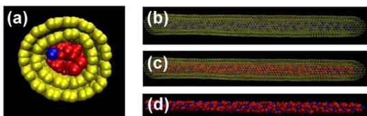
**Figure 1.** Snapshots of the simulated systems containing CNTs. Cations are red balls, anions are blue balls, CNT atoms are in yellow. The snapshots were taken after the filling had been finished. (A) top view of CNT-10; (b) packing of chloride anions in CNT-10, side-view; (c) CNT-13, side view, nanotube atoms are shown as wires to make ions visible; (d) CNT-13, side view, nanotube atoms are omitted for clarity.
