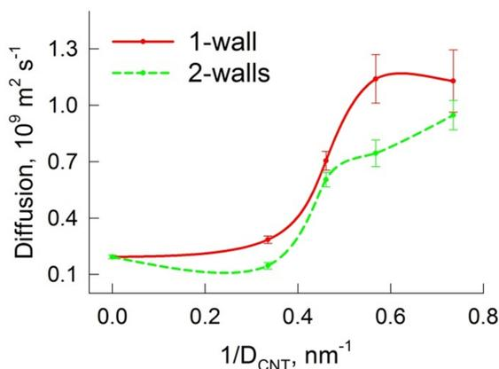
**Figure 5.** Diffusion of  $[C_2C_1IM][Cl]$  inside double-walled carbon nanotubes in the CNT-10, CNT-13, CNT-16, CNT-19, CNT-22, and BULK systems. The depicted values are averaged over all cations and anions. Therefore, these values reflect the total mobility of ions in the investigated systems.
