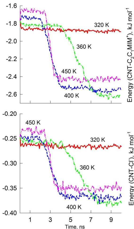
**Figure 3.** Pairwise interaction energy between  $[\text{C}_2\text{C}_1\text{IM}]^+$  cations and CNTs (top panel); between  $[\text{Cl}]^-$  anions and CNTs (bottom panel) during CNT filling at various temperatures (320, 363, 400, 450 K). Filling of CNT-10 was investigated, as the most interesting case.
