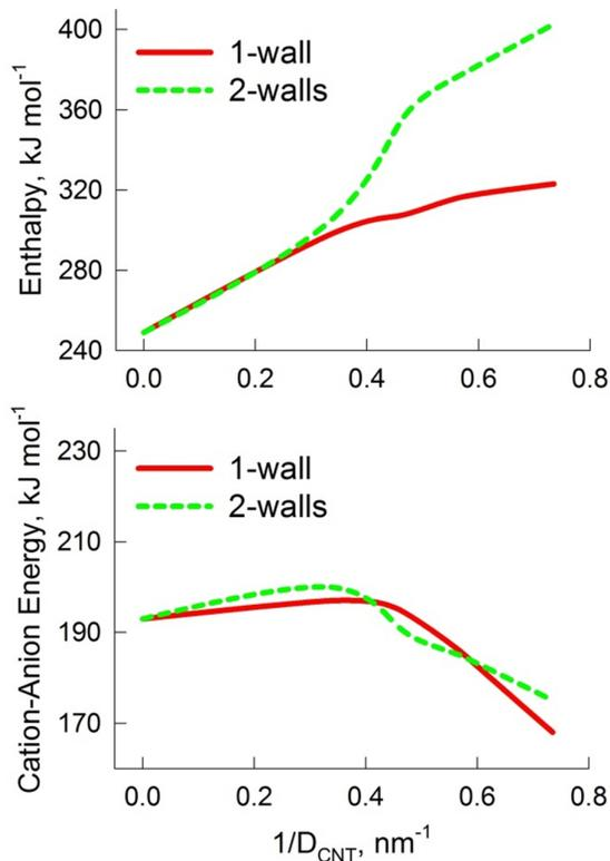
**Figure 6.** (Top panel) Enthalpy corresponding to a single IL ion pair versus CNT diameter and in bulk  $[\text{C}_2\text{C}_1\text{IM}][\text{Cl}]$  ( $1/D_{\text{CNT}} = 0$ ). (Bottom panel) Pairwise ion interaction energy versus CNT diameter and in bulk. Both enthalpy and pairwise ion interaction energy are represented as absolute values for clarity.
