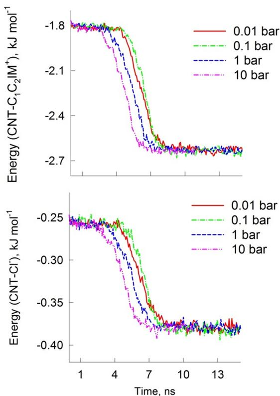
**Figure 4.** Pairwise interaction energy between  $[\text{C}_2\text{C}_1\text{IM}]^+$  cations and CNTs (top panel); between  $[\text{Cl}]^-$  anions and CNTs (bottom panel) during CNT filling at various external pressures (0.01, 0.1, 1, 10 bar). Filling of CNT-10 was investigated at 363 K, as the most interesting case.
