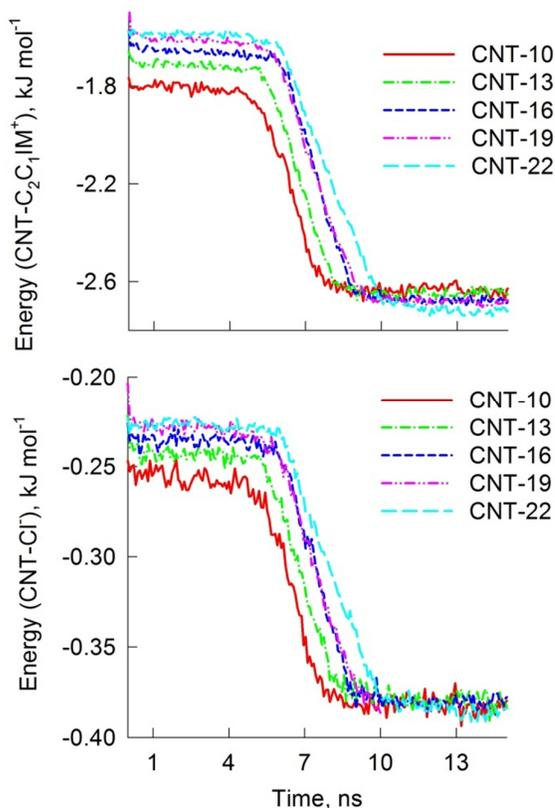
**Figure 2.** Pairwise interaction energy between  $[\text{C}_2\text{C}_1\text{IM}]^+$  cations and CNTs (top panel); between  $[\text{Cl}]^-$  anions and CNTs (bottom panel) during CNT filling, conducted at 363 K.
