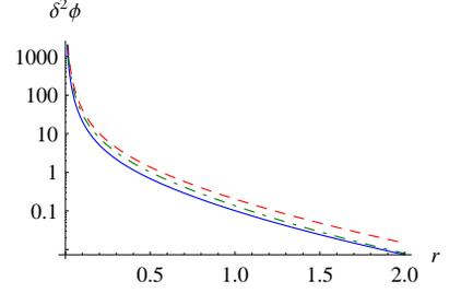
FIG. 1: The plots of  $\delta^2\phi$  versus the squeeze parameter  $r$  for the TMSV inserted before (solid) and after (dashed/dot-dashed) the first BS. Here the average excitation number  $N = 0.2$ . The transmissivity of light beam  $\epsilon_1 = 0.8$ ,  $\epsilon_2 = 0.8/1.0$  (dashed/dot-dashed).
