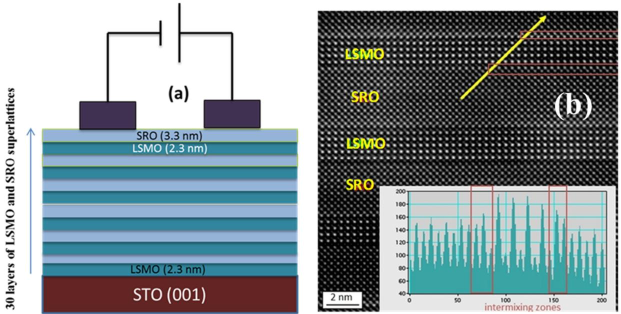
**Fig. 1:** (a) Schematic of device that was made using  $\text{La}_{0.7}\text{Sr}_{0.3}\text{MnO}_3$  (LSMO)/  $\text{SrRuO}_3$  (SRO) superlattice. The superlattice consist of 30 layers of LSMO (2.3 nm) and SRO (3.3 nm) deposited on  $\text{SrTiO}_3$  (001), as shown in the schematic. (b) HAADF-STEM micrograph of the  $\text{La}_{0.7}\text{Sr}_{0.3}\text{MnO}_3$  /  $\text{SrRuO}_3$  superlattices: the brown rectangles indicate the interfacial regions that are affected by intermixing.
