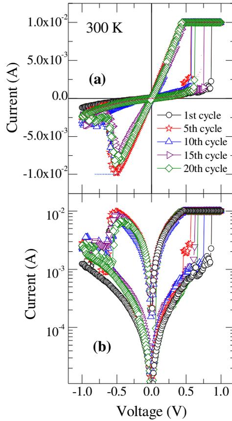
**Fig. 2:** Bipolar resistive switching characteristics of LSMO/SRO superlattice at room temperature (300 K) . **(a)** I – V characteristics indicates that the current switching behavior is quite stable. **(b)** Shows the same graph in logarithmic plot
