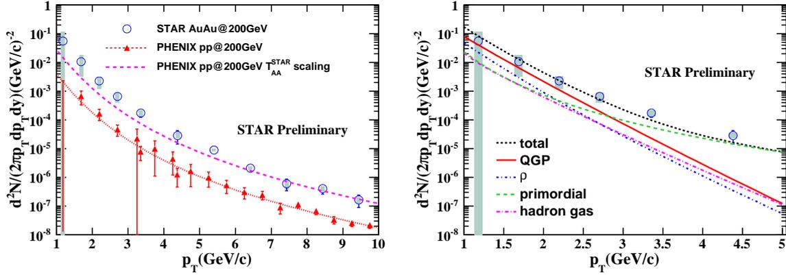
Figure 3. Left panel shows the direct photon invariant yield. The pink dashed curve represents a power-law fit to PHENIX 200 GeV  $p + p$  cross section [14, 16], scaled by  $T_{AA}$ . Right panel shows the direct photon invariant yield compared to model predictions including the contributions from different sources [5, 18]. The statistical and systematic uncertainties are shown by the bars and bands, respectively.
