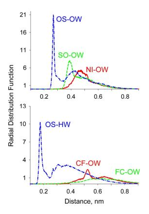
Figure 3. Radial distribution functions for the selected sites of the TFS $\Gamma$  anion and surrounding water molecules. Atom names in the legends are used as in common empirical force fields: OS – oxygen of TFS $\Gamma$ ; SO – sulfur of TFS $\Gamma$ ; NI – nitrogen of TFS $\Gamma$ ; CF – carbon in trifluoromethyl group of TFS $\Gamma$ ; FC – fluorine in trifluoromethyl group of TFS $\Gamma$ ; OW – oxygen of water; HW – hydrogen of water.
