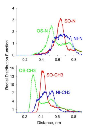
Figure 4. Radial distribution functions for the selected sites of the TFS $\Gamma$  anion and surrounding acetonitrile molecules. Atom names in the legends are used as in common empirical force fields: OS – oxygen of TFS $\Gamma$ ; SO – sulfur of TFS $\Gamma$ ; NI – nitrogen of TFS $\Gamma$ ; CF – carbon in trifluoromethyl group of TFSI $\Gamma$ ; FC – fluorine in trifluoromethyl group of TFSI $\Gamma$ ; N – nitrogen of ACN; CH<sub>3</sub> – carbon of methyl group.
