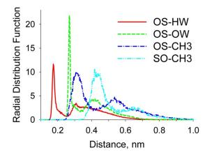
Figure 5. Competitive solvation of the TFSI<sup>-</sup> anion by water and acetonitrile molecules in terms of radial distribution functions. Atom names in the legends are used as in common empirical force fields: OS – oxygen of TFSI<sup>-</sup>; SO – sulfur of TFSI<sup>-</sup>; OW – oxygen of water; HW – hydrogen of water; CH<sub>3</sub> – carbon of methyl group.
