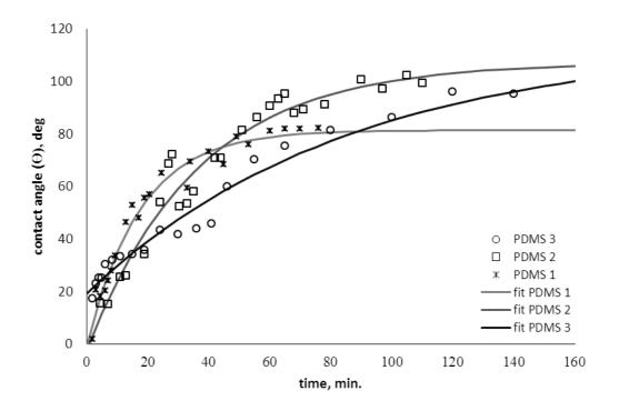
Fig. 6. The apparent contact angle (APCA)  $\theta^*$  as a function of the time, *t*. Solid lines depict the exponential fitting of experimental data with Exp. 2.
