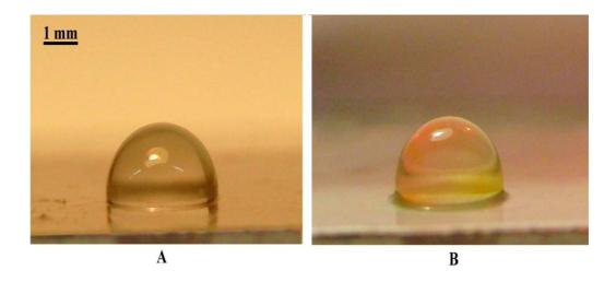
Fig. 4. A. 8 μl water droplet coated with a layer of the non-colored silicone oil.B. 8 μl water droplet coated with a layer of the silicone oil, colored with the orange pigment.
