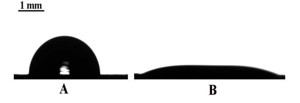
Fig. 5. 8 µl water droplet deposited on non-treated (A) and plasma-treated (B) PDMS1 silicone oil.
