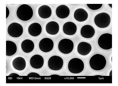
Fig. 1. Polycarbonate honeycomb coating of Al foil obtained with "breath-figures", carried out in a humid atmosphere. Scale bar is 1  $\mu$ m.
