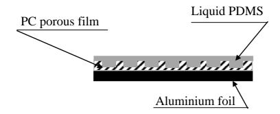
Fig 2. Scheme of PDMS oil layers exposed to air plasma discharge.
