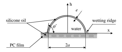
Fig. 3. Wetting regime for water droplets deposited on the silicone oil layer.  $\theta^*$  is the apparent contact angle.
