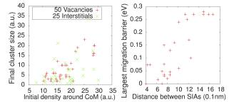
FIG. 4. Left panel: the size of the clusters in the final configuration after the 50-vacancy ( $R^2=0.58$ ) and 25-SIA ( $R^2=0.14$ ) simulations as a function of the initial density of point defects in the neighborhood of their CoM. Right panel: The largest barrier crossed when two SIAs set at a given distance from each other aggregate ( $R^2=0.69$ ).
