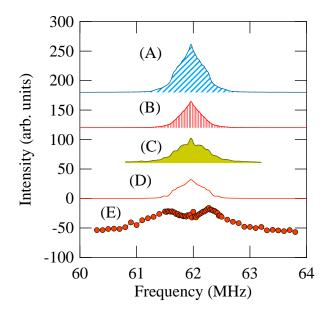
FIG. 5. <sup>209</sup>Bi powder spectra simulated by three separate methods, (A), (B), and (C), as described in the text. (D) Sum of theoretical amplitude spectra with the same number of angle points as the experimental data; this spectrum exhibits bumpiness similar to the solid gold pattern. (E) Experimental spectrum of mortar-and-pestle ground sample.
