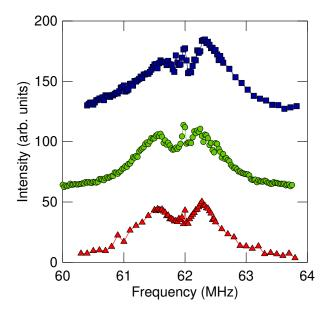
FIG. 4. Experimental 10 K, 9 T  $^{209}$ Bi spectra of Bi<sub>2</sub>Se<sub>3</sub> ground with a mortar and pestle, showing the spectrum of bulk states. The data was first taken with the powder asmade (blue squares), then after strain relief (green circles), then after fixing in epoxy resin in zero field to prevent alignment of grains (red triangles). All three spectra are dominated by two broad peaks, as in the nanoparticle case (Fig. 3).
