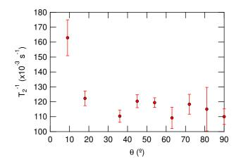
FIG. 8. Spin-spin relaxation rate as a function of angle for single crystal of  $Bi_2Se_3$ . The relaxation times are independent of angle above  $18^\circ$ , thus ruling out spin-spin decoherence as a cause for the anisotropy of signal intensity.
