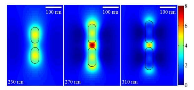
**Figure.S1: FDTD simulation of enhancement effects of two-wire antennas with three different sizes: 230, 270 and 310 nm.** The enhancement is shown as the field intensity at the middle of TbFeCo layer normalized by the case without antennas. White bar at top right corner is 100 nm in length.
