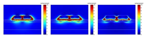
**Figure S2 | FDTD simulation normal to the sample plane of enhancement effects of the twowire antennas with three different sizes: 230, 270 and 310 nm.** The enhancement is shown for the field intensity at the middle of the respective antennas normalized by the case without antennas.
