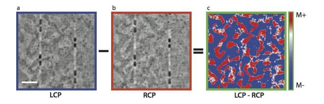
**Figure 3 | Separating magnetic and non-magnetic image contrast. a, b**, Individual holographic image reconstructions obtained with LCP (left) and RCP (middle) x-rays at 706.8 eV, show a superposition of magnetic domains and the antenna structures. The white scale bar in figure **a** is 400 nm in length. **c**, The difference image (right), LCP – RCP, reveals the magnetic domain structure. A multi-domain magnetic structure was prepared by using an incident laser fluence of 21 mJ/cm<sup>2</sup>.
