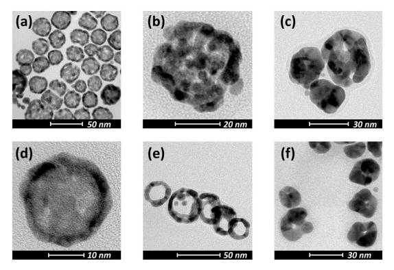
**Figure 1.**(*a*) – (*c*) Conventional TEM images characteristic of samples of aqueous dispersions of HGNPs at different pHs: 7, 5 and 2, respectively. pH modification was achieved by adding increased amounts of HCl. (*d*) – (*f*) Conventional TEM images characteristic of samples of aqueous dispersions of 1:1 Poly-L-Lysine Hydrobromide: HGNPs (0,5 mg/mL), corresponding to (*d*) initial, (*e*) after 2 h of reaction time (pH = 5) and (*f*) after 28 h of reaction time (pH = 5).
