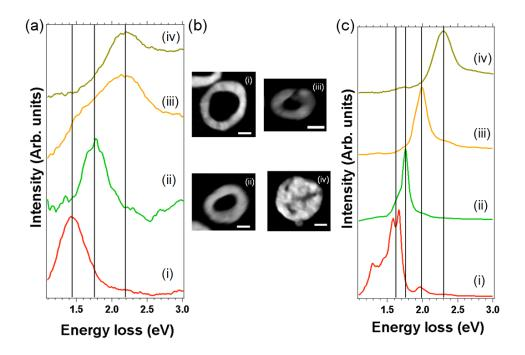
**Figure 4.** (a) EEL spectra (each of them corresponds to the sum of 8-12 spectra, after background subtraction) recorded on nanorings of different aspect ratios ( $\sigma$ ), (see table) ring 1 (i), ring 3 (ii), ring 6 (iii) and hollow sphere (iv). (b) HAADF images of the corresponding nanostructures. Scale bar is 10 nm for all these micrographs. (c) EELS DDA simulations for the corresponding (same sizes) NPs.
