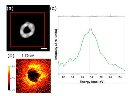
*Figure 3. (a)* HAADF-STEM image (scale bar 10 nm) of an Au nanoring, where an EELS SPIMs has been recorded in the red marked area. (b) Intensity maps showing the spatial distribution of the SPR mode (1.75 eV.) for this Au NR. (c) EEL spectrum, after background subtraction, corresponding to the sum of 12 spectra. .
